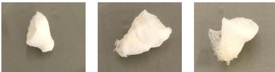
Figure 4. 19. Biofoams produced by using high molecular weight chitosan (a) 1 % HMW CS, 10 volume % hexane, (b) 1 % HMW CS, 13 volume % hexane (c) 1 % HMW CS, 17 volume % hexane.
