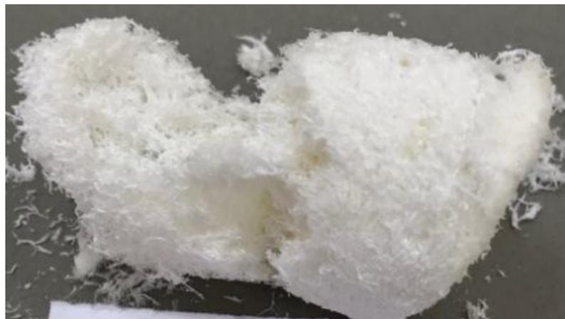
Figure 4. 17. Produced foam by using O/W spontaneous emulsion templated method.
