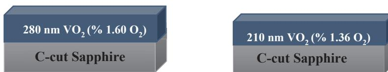
Figure 3.1. Schematic representation of VO<sub>2</sub> thin films on c-cut sapphire substrate with different thickness and oxygen concentration.
