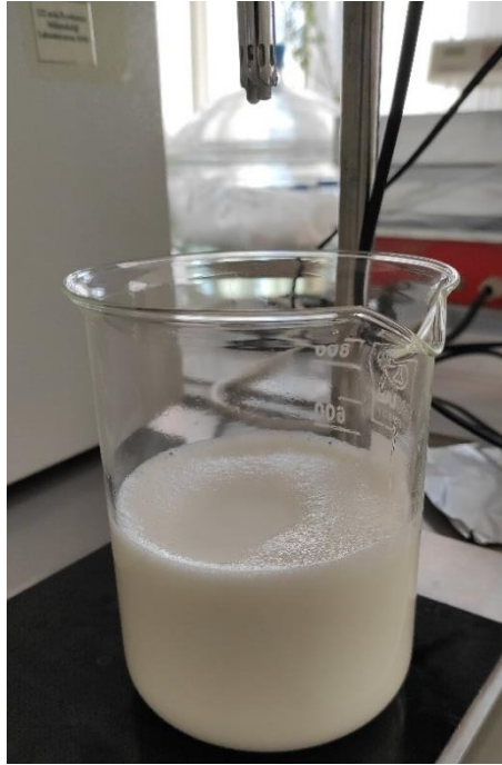
Figure 3.9: The sample of blended emulsion fuel at the end of the preparation process
