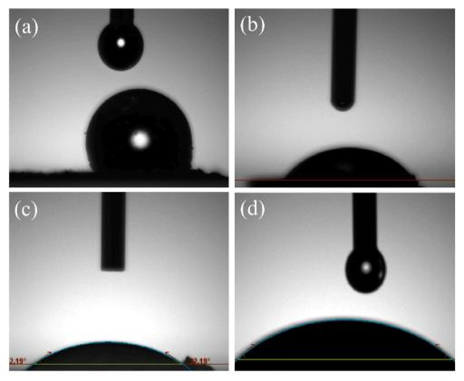
Fig. 3. Wetting angle test results; (a) NB600 CA [°]:114 ± 40, (b) NB1200 CA [°]:27 ± 10, (c) NB600Ti CA [°]: 32 ± 0.2, and (d) NB1200Ti CA [°]: 38 ± 0.2.
