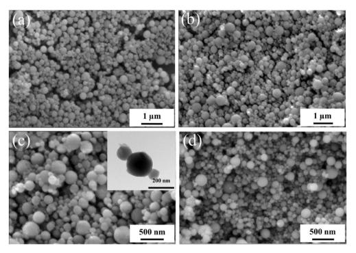
Fig. 1. SEM images of the formed samples; (a) polymeric NBs, (b) sample pyrolyzed at 600 °C: NB600, (c) higher magnification image of NB600 (the inset shows the TEM images of NB600), and (d) sample pyrolyzed at 1200 °C: NB1200.
