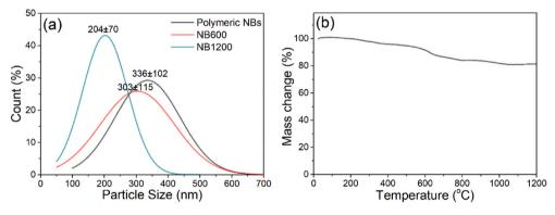
Fig. 2. (a) Particle size (diameter) distributions of polymeric NBs, and samples obtained by the pyrolysis at 600 and 1200 °C for 2 h at peak temperature, (b) TGA analysis of the polymeric NBs taken with 5 °C/min; N<sub>2</sub> flow 0.05 L/min.
