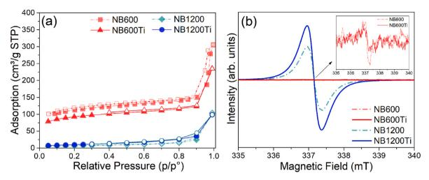
Fig. 5. (a) N<sub>2</sub> sorption isotherms, and (b) X-band EPR spectra of the bare and TiO<sub>2</sub>-coated NBs.
