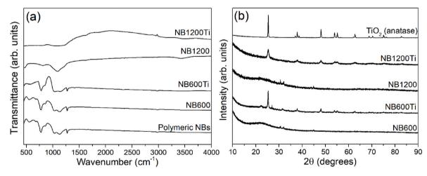
**Fig. 4.** Normalized; (a) FTIR spectra of polymeric, pyrolyzed and TiO<sub>2</sub>-coated NBs, and (b) XRD patterns of bare and TiO<sub>2</sub>-coated ceramer and SiOC NBs produced by 600 °C, and 1200 °C pyrolysis. At the top of the experimental data, reference reflection marks for pure anatase TiO<sub>2</sub> (ICDD PDF #00-021-1272) are given.
