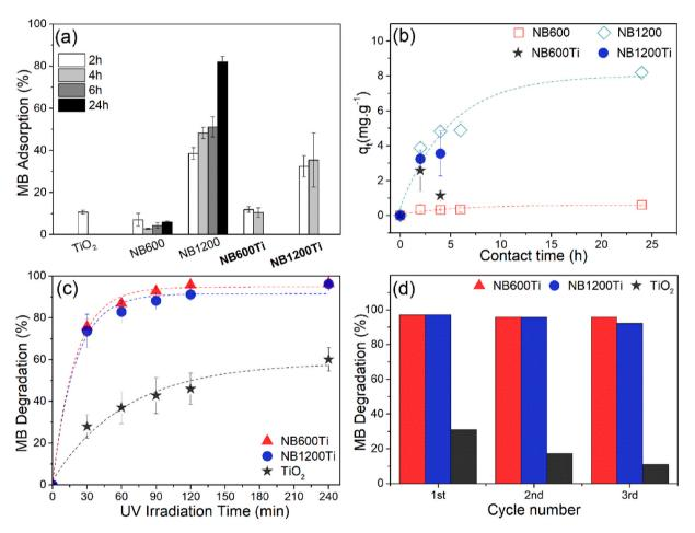
**Fig. 6.** (a) MB adsorption efficiency in the dark with different contact times for NB600, NB1200, NB600Ti, NB1200Ti, and  $TiO_2$  powder, (b) effect of contact time on MB adsorption capacity for uncoated and  $TiO_2$ -coated NBs, (c) MB degradation efficiency under UV light irradiation for NB600Ti, NB1200Ti, and  $TiO_2$  powder (the dashed lines represent the exponential non-linear fitting resulting with  $R^2 > 0.7370$ ), and (d) reusability of the photocatalyst.
