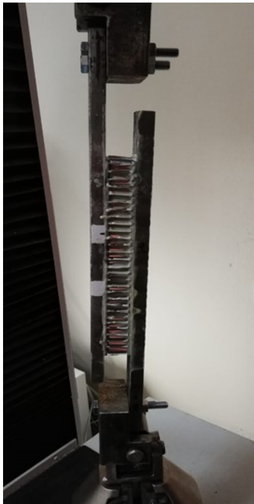
Figure 4.1. Core shear test set-up with special testing apparatus according to ASTM C273
