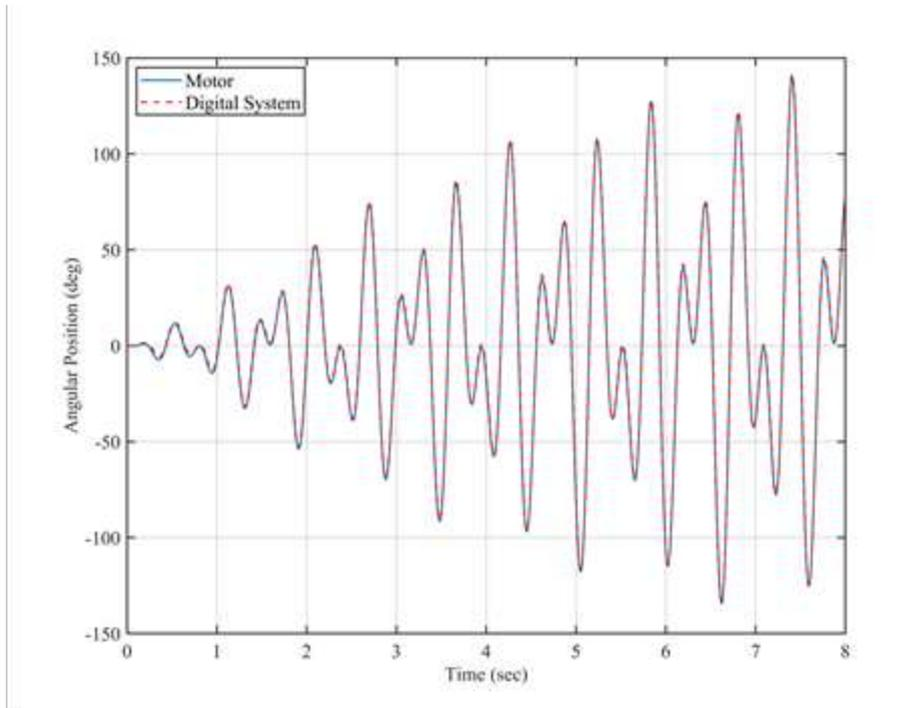
Fig. 5 Response of both the actual system and its DT for a random input
