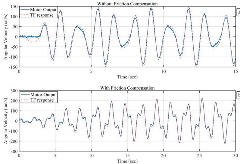
**Fig. 4.** TF (red) and servo motor's measured (blue) outputs when (a) there is no friction compensation. (b) there is friction compensation.
