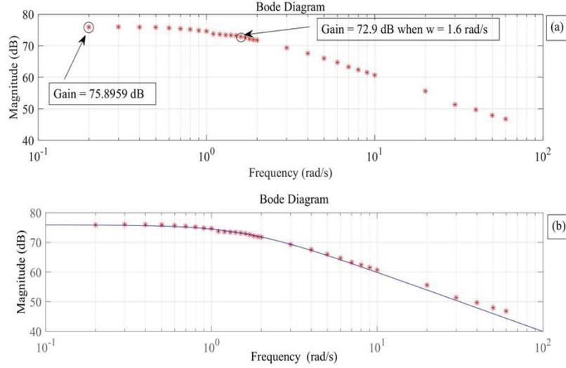
**Fig. 3.** Experimental results for identifying the current-controlled servo motor system (a) Measured Data (red) (b) Bode Diagram of the fitted TF (blue) and measured data (red).
