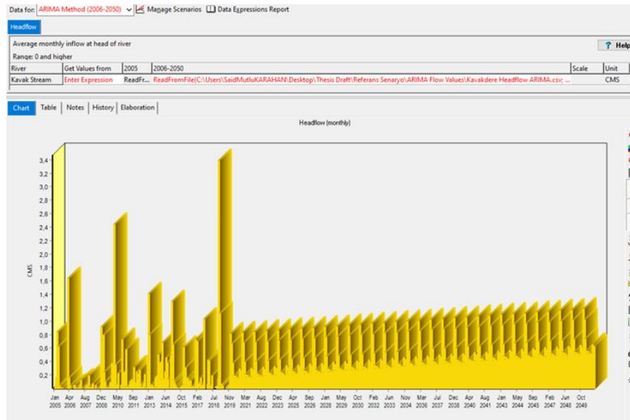
Figure 6.52. Forecasted Flow Values of Kavakdere Stream Under Autoregressive Integrated Moving Average Method
