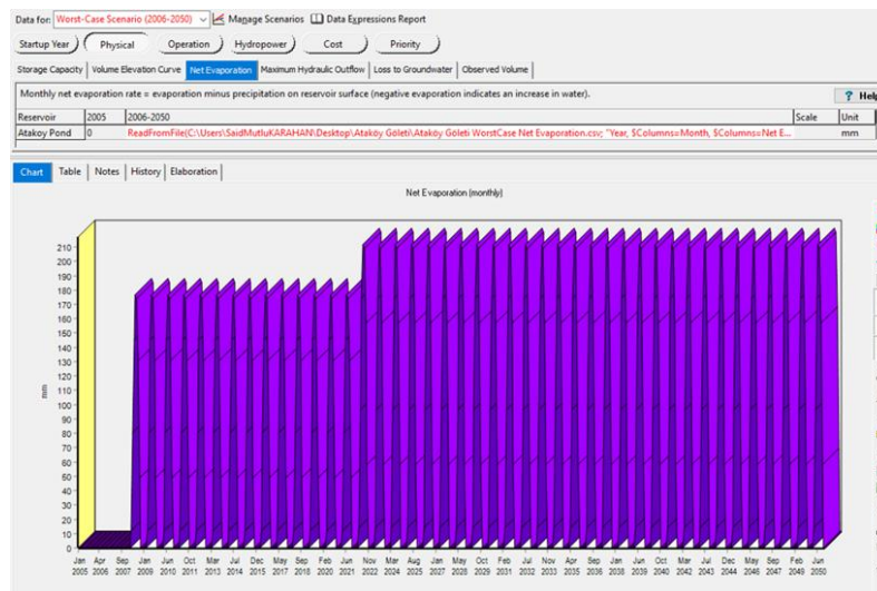
Figure 6.37. Net Evaporation Values of Ataköy Pond in the Worst Case Scenario (mm)
