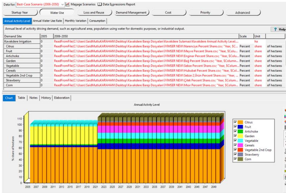
Figure 6.33. Kavakdere Dam Irrigation Changing Crop Pattern
