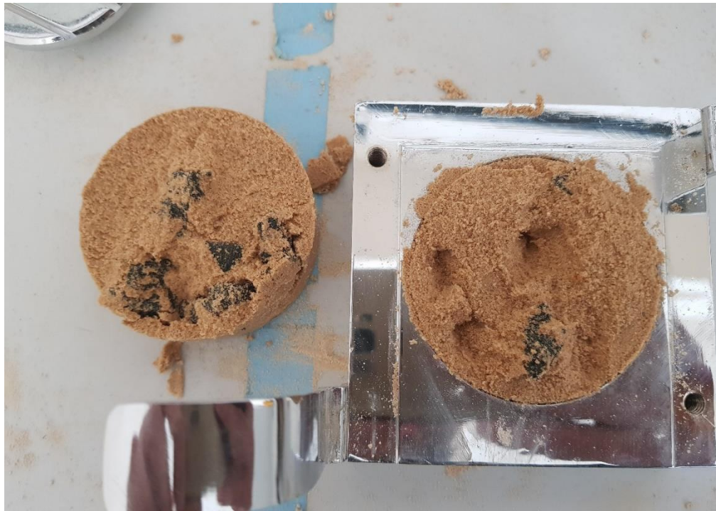
Figure 5.5. Tested sample shows the coarse granulated rubber distribution in the sand-granulated rubber mixture.
