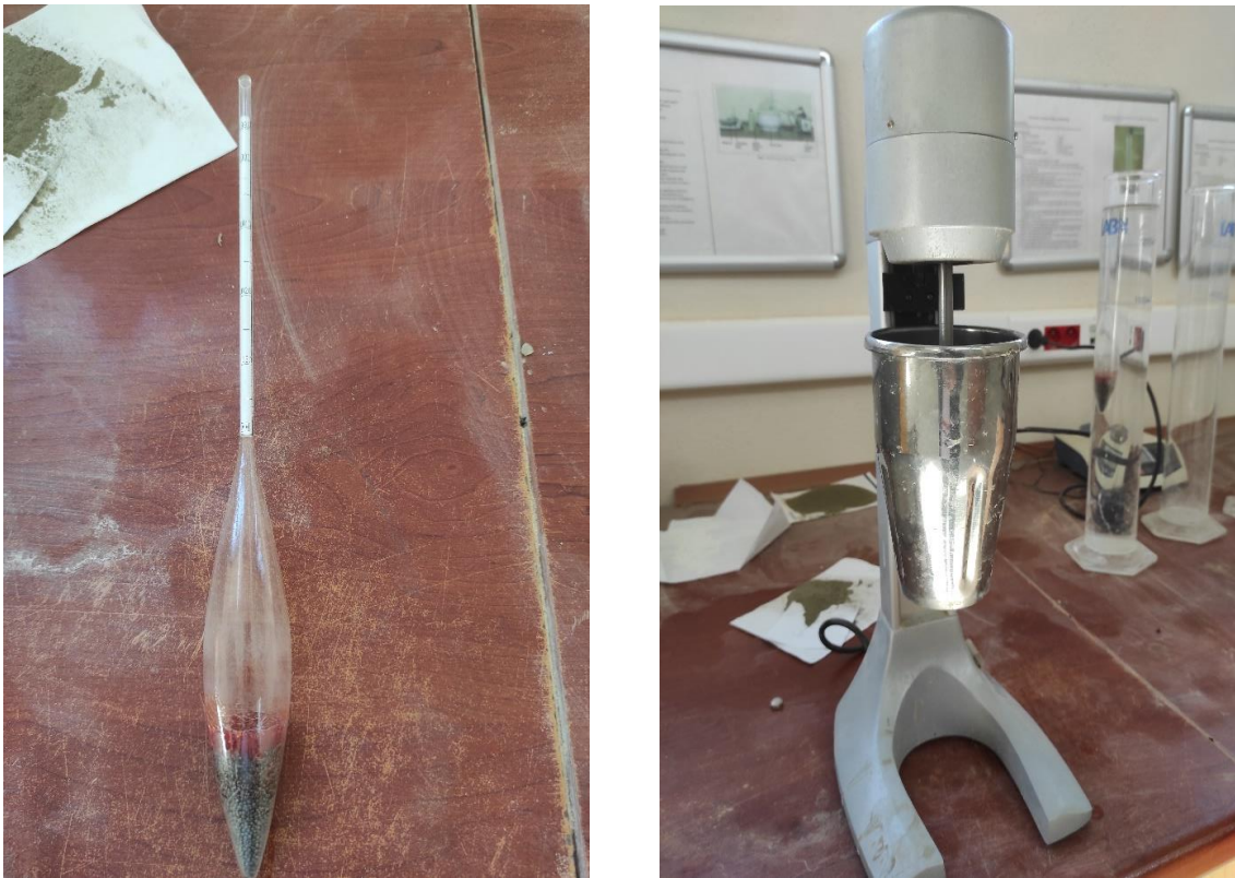
Figure 3.3. An equipment used for the hydrometer test; (a) hydrometer, and (b) sample mixer
