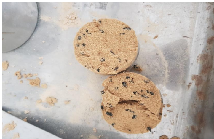
Figure 5.1. Tested sample shows the fine granulated rubber distribution in the sand-granulated rubber mixture.
