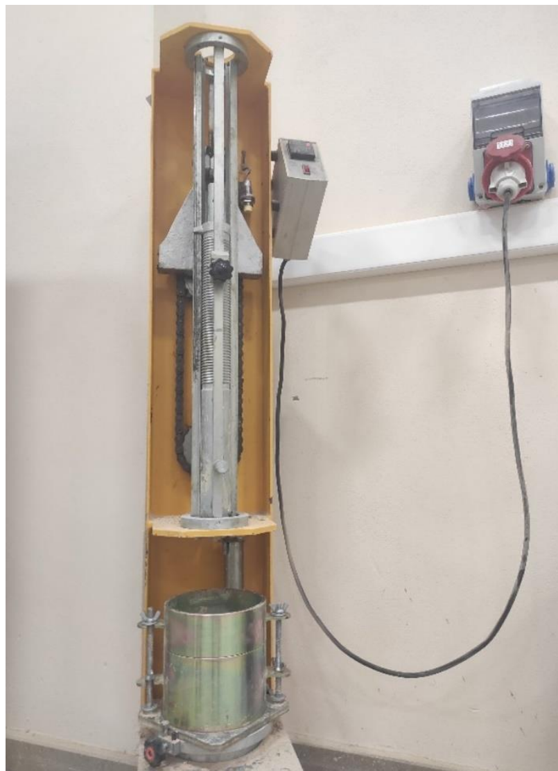
Figure 3.5. Mechanical compacter and C type mold
