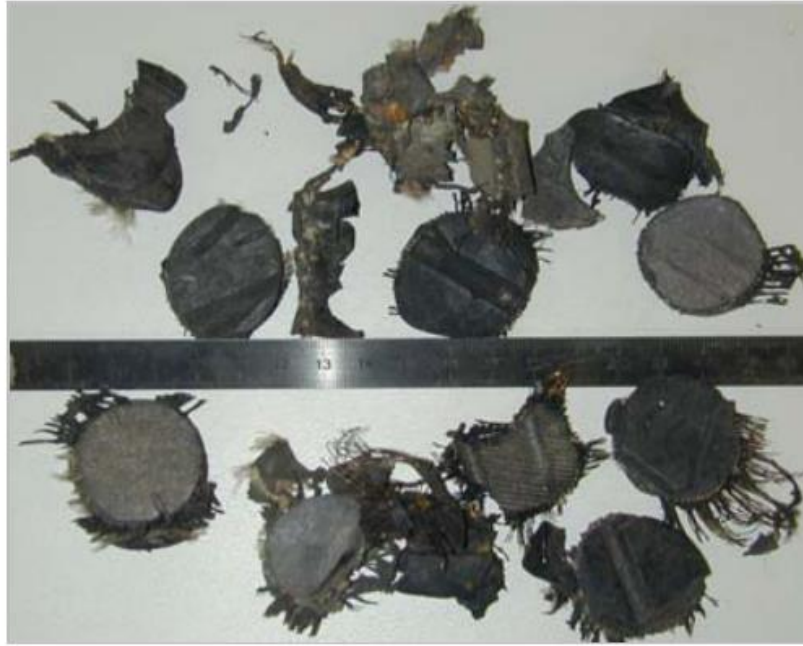
Figure 2.1. Tire chips that used in the study (Source: Lambert, Bałachowski, and Gotteland, 2005)
