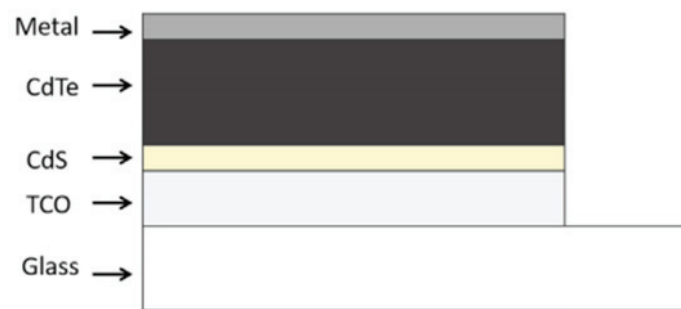
Figure 2.2. Typical CdTe solar cell structure. (Source: Baines et al. 2018)
