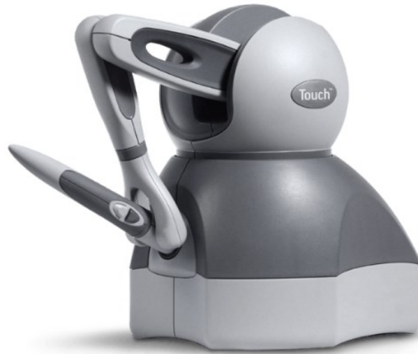
Figure 3.3 Geomagic Touch™ haptic device.
