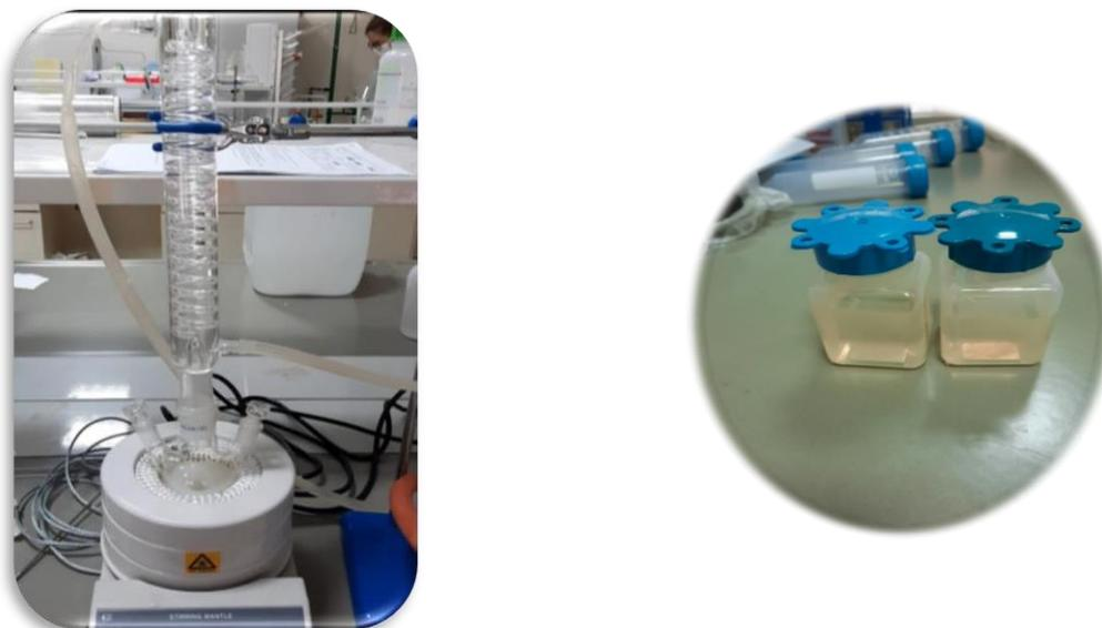
Figure 4.1 Experimental Set-up and biolubricant obtained
