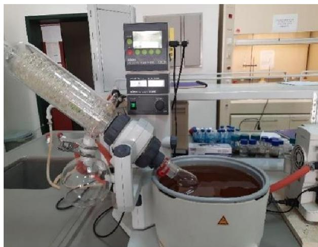
Figure 4.2. Removal of excess alcohol with rotary evaporator
