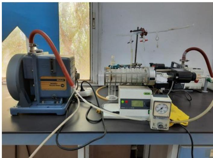
Figure 4.3. Removal of excess alcohol with Kugel vacuum distillation
