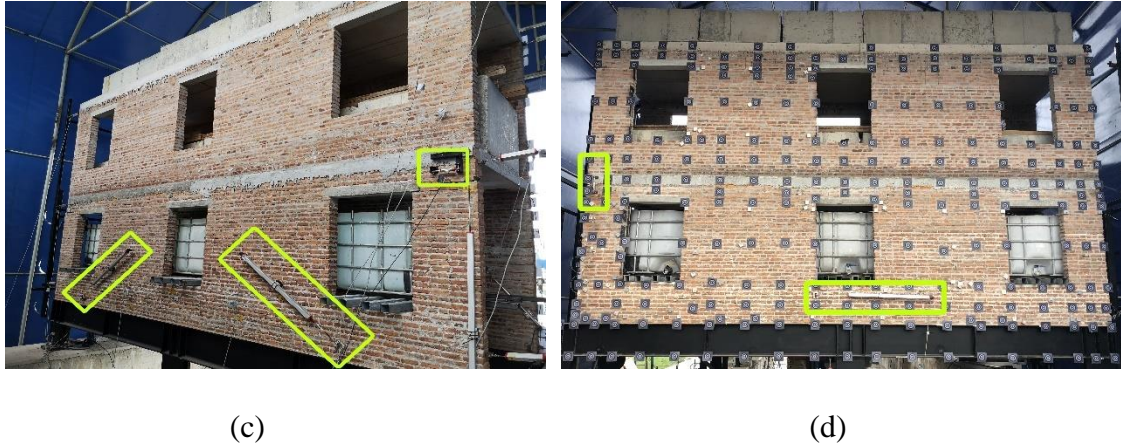
Figure 3.10. LVDT's installed to measure: (a) horizontal displacements, (b) vertical displacements, (c) & (d) local crack openings and sliding.
