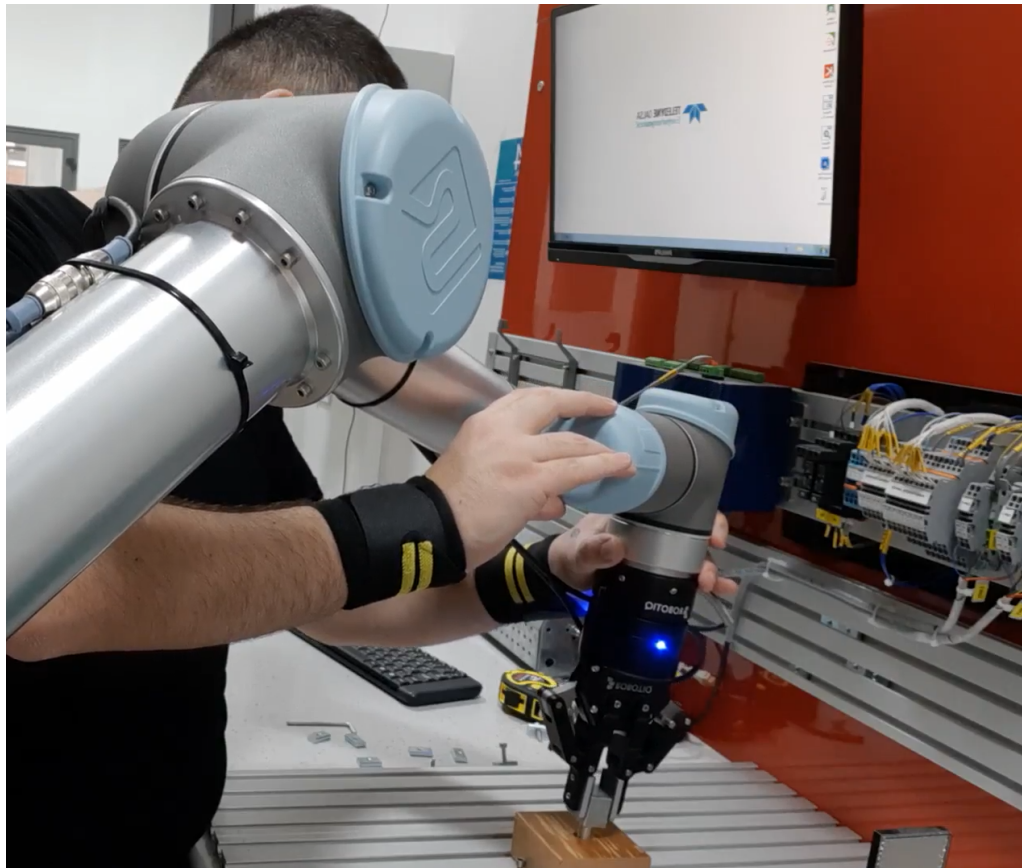
Figure 3.4. Kinesthetic teaching of the peg-in-hole task.
