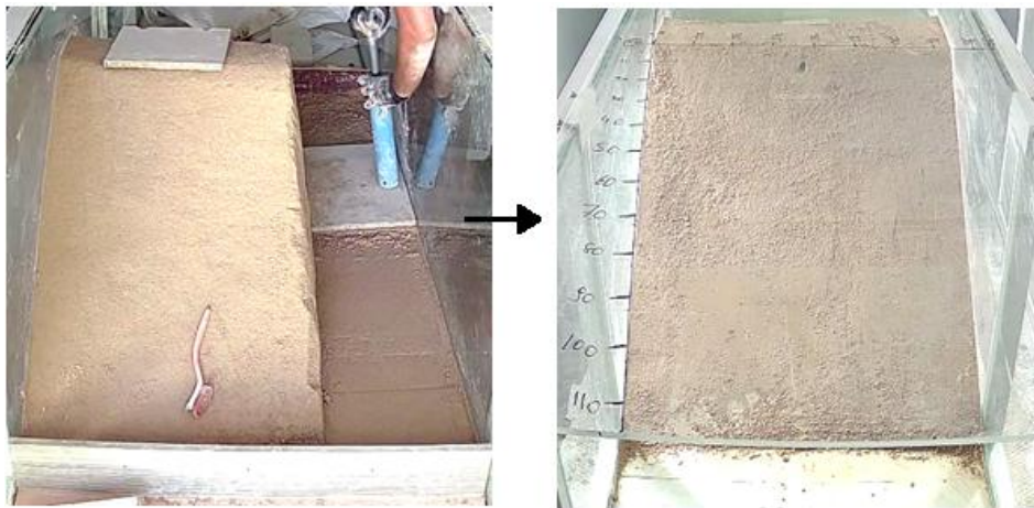
Figure 5.6 Construction of the trimmed part to create the dam for the second scenario
