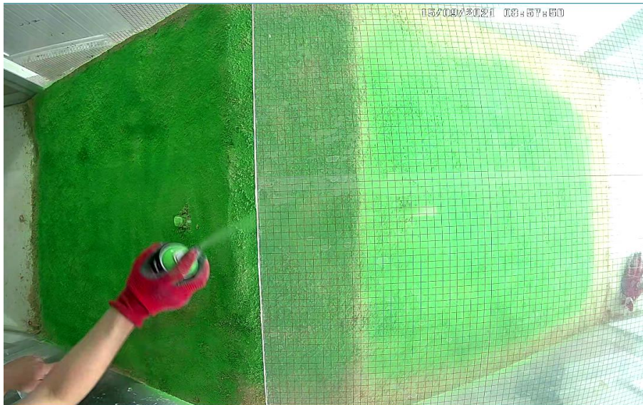
Figure 5.9 Painting the dam surface with green spray for the third scenario
