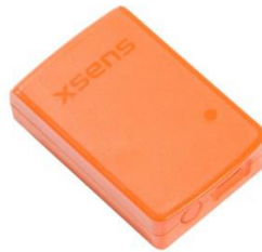
Figure 2: Front side of the MTw (motion tracker) [31]
