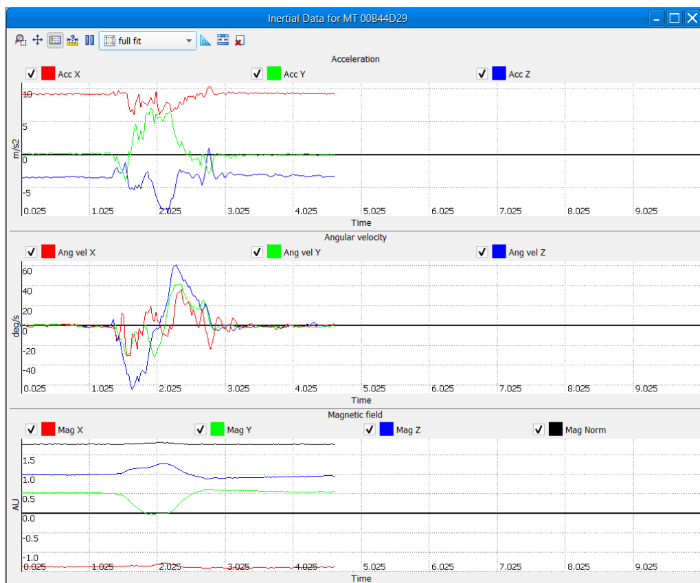
Figure 11: Inertial data graph of the player 4’s first dig recorded by left leg sensor (sensor 1)
