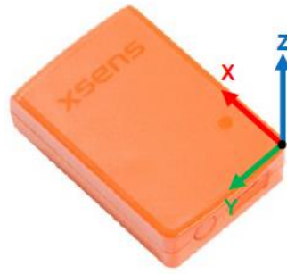
Figure 4: The object coordinate system [31]
