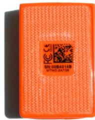
Figure 3: Rear side of the MTw (motion tracker) where MTw product code (MTW2 – 3A7G6) and serial number (device id) are visible for the user to simply identify each MTW's [31]
