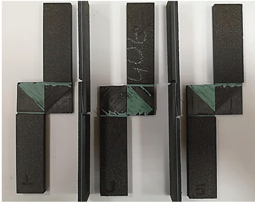
Figure 3. 20. Single lap shear reference test specimen after environmental aging
