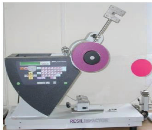
Figure 2. 13. Test set-up for the charpy impact test.
