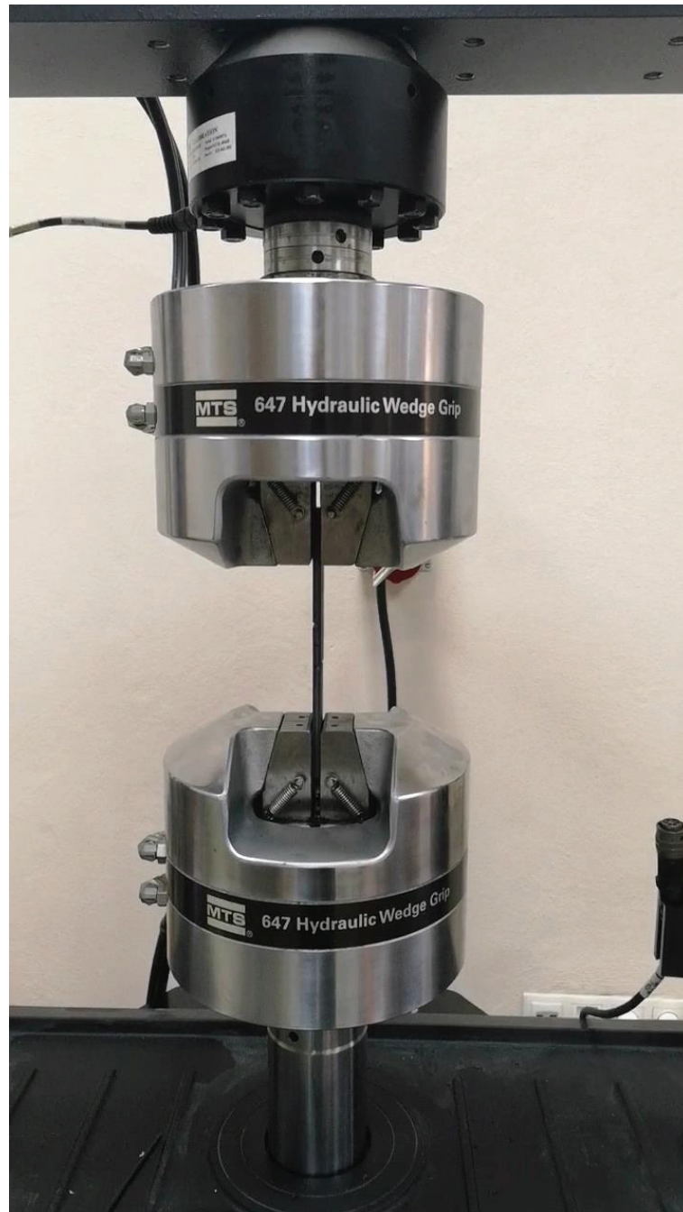
Figure 2. 11. Test set-up for the single-lap joint.
