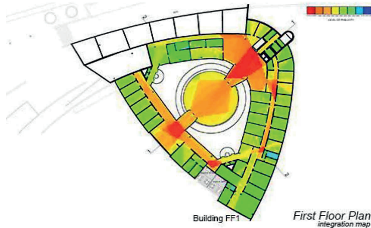
Figure 17. Karabük Municipality Service Building Competition, First Prize, Integration map of first floor plan
