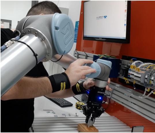
Fig. 1. Demonstrations are performed using a UR5 manipulator
