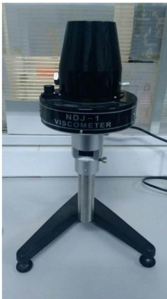
Figure 3. 3. The experimental setup for viscosity measurement of precursor inks.
