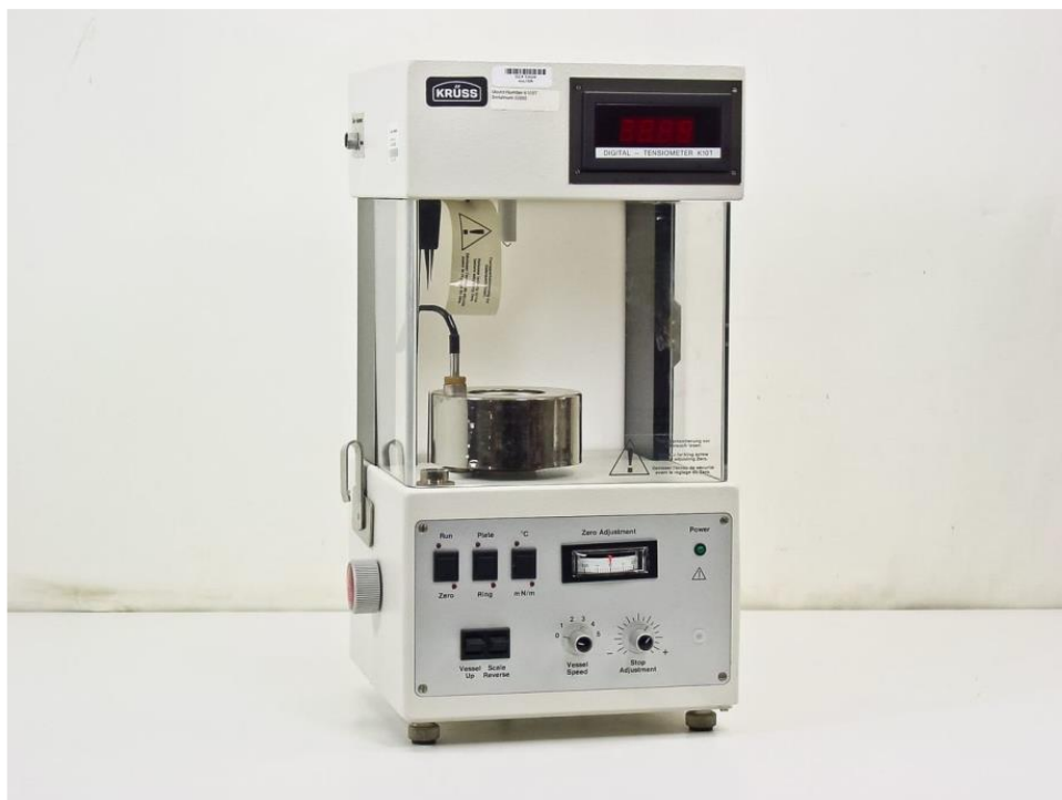
Figure 3. 4. The experimental setup for surface tension measurement of precursor inks.
