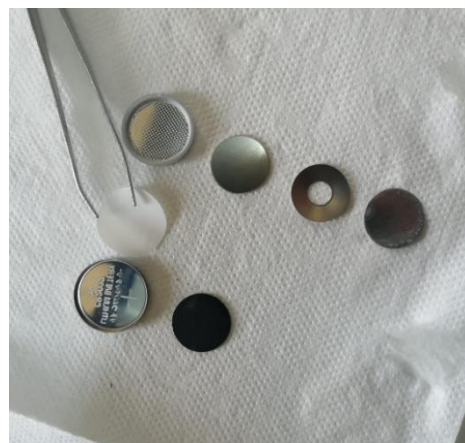
Figure 2.4. Coin cell components
