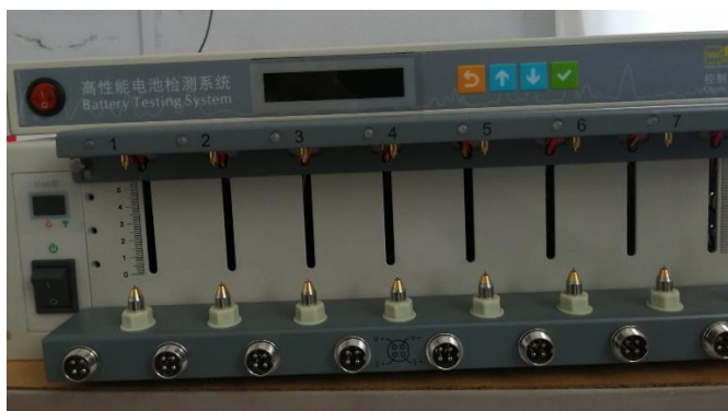
Figure 2.6. BTS CT-4008T battery tester
