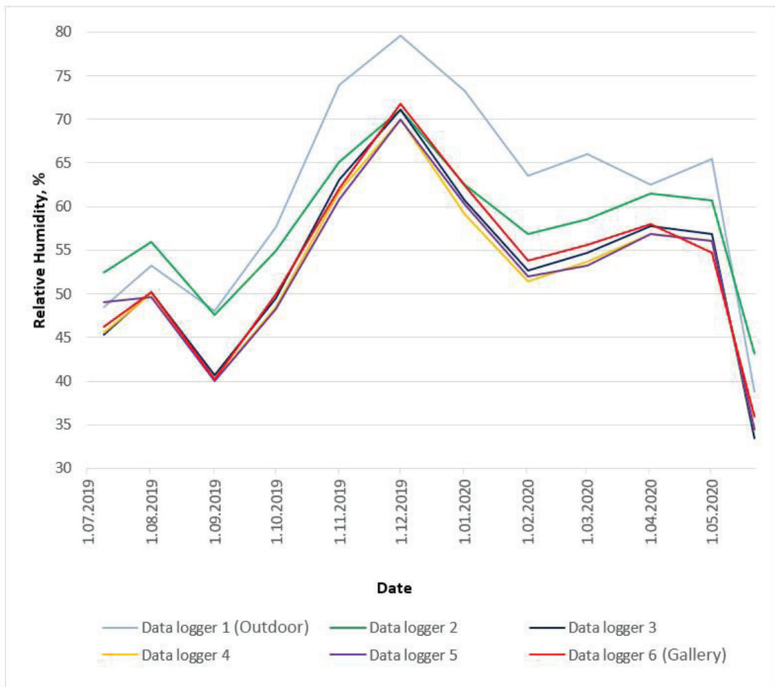
Figure 5.14. Comparison of monthly relative humidity values measured by six devices
