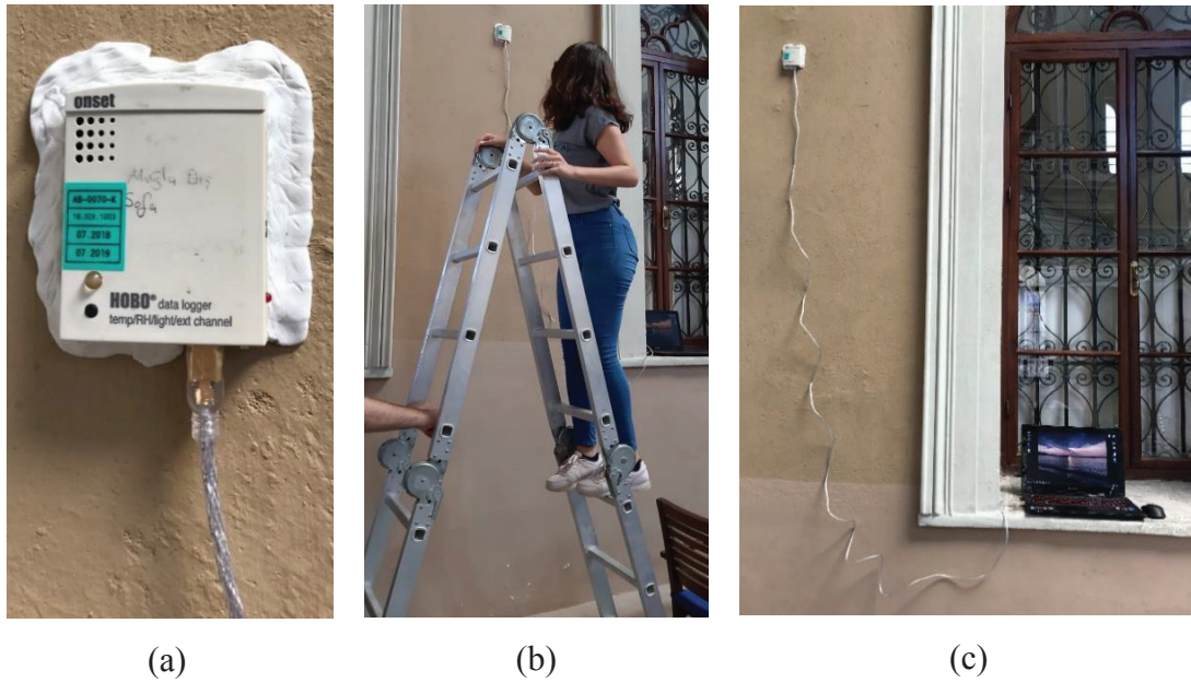
Figure 3.4. Data transfer from data logger No. 2 to digital environment (07.08.2019), a) Data logger No. 2, b) Attaching a connecting cable to the device, c) Data transfer
