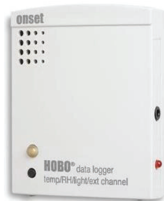
Figure 3.1. HOBO U12-012 data logger device (Source: Onset, 2019)
