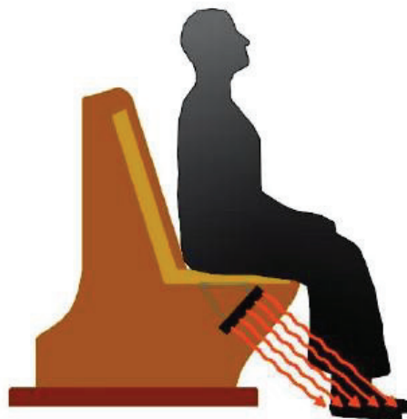
Figure 5.32. Pew heating by using low temperature radiant heaters (Source: Pałupska and Kanaś, 2018)
