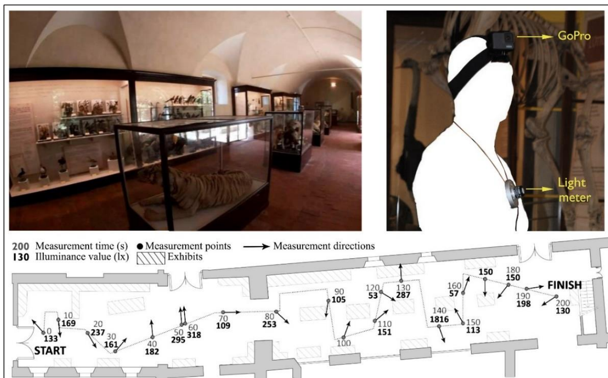
Figure 2. A still from videos (top left); the placement of camera and luxmeter (top right); and illuminance measurements and directions marked on the floor plan for Room A (bottom).
