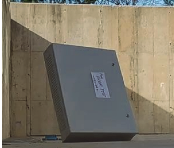
Figure 29. Drop test for edge
