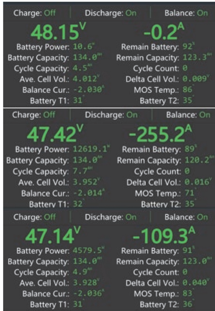
Figure 55. BMS voltage and ampere result
