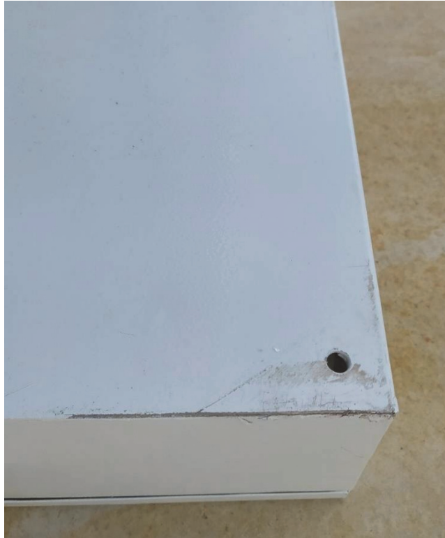
Figure 51. Drop test result for edge
