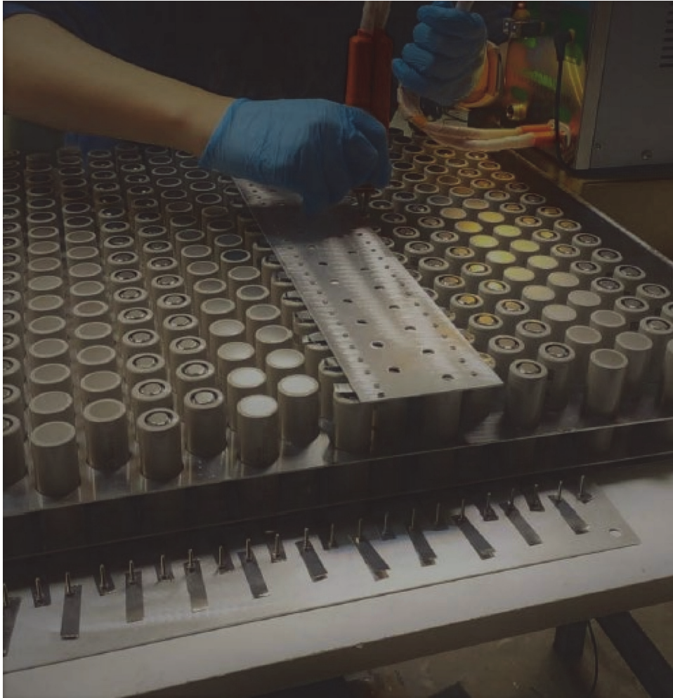
Figure 47. Welding nickel strips to battery cell with Spot welding
