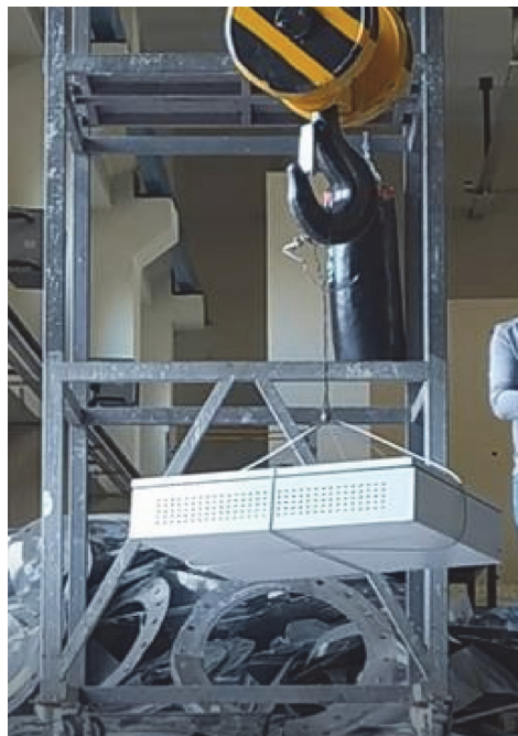
Figure 28. Drop test for base plate
