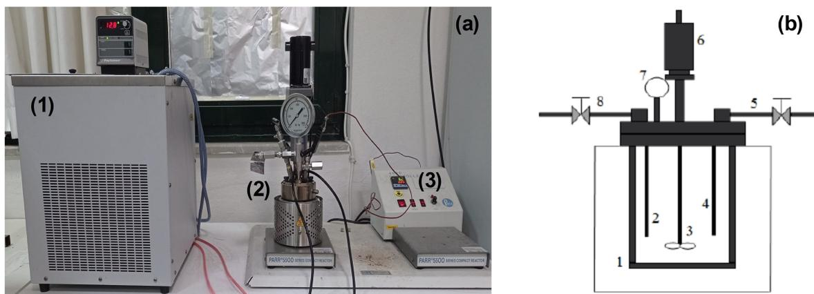
**Figure 6.** (a) Experimental Setup for subcritical wastewater treatment: (a-1) Chiller, (a-2) Batch reactor, (a-3) Heater; (b) Batch reactor for hydrothermal liquefaction of sugar industry wastewater: (b-1) stainless steel beaker, (b-2) thermocouple, (b-3) stirring impeller, (b-4) gas inlet, (b-5) input nitrogen gas, (b-6) magnetically driven stirrer, (b-7) pressure gauge, (b-8) gas sample collecting valve.
