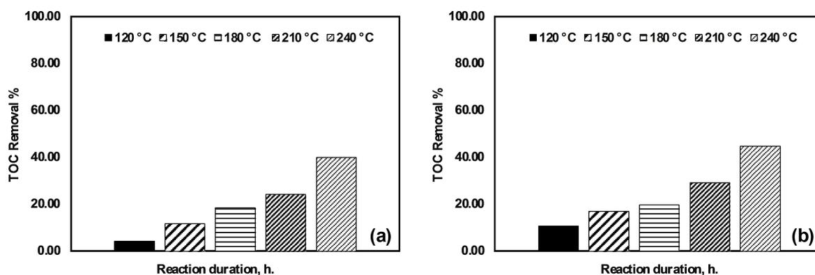
Figure 1. TOC removal % depending on reaction duration 1 h (a) and 2 h (b) (reaction conditions: 100 ml of sugar industry wastewater,  $T = 120\text{--}240\text{ }^\circ\text{C}$ ,  $t = 1\text{--}2\text{ h}$ ).
