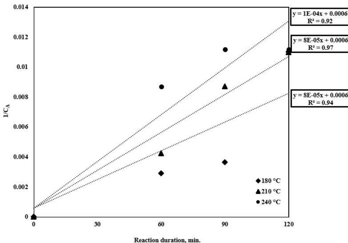
Figure 4. Linearized second-order kinetic plot (reaction conditions: 100 ml of sugar industry wastewater,  $T = 180, 210,$  and  $240^\circ\text{C}$ ,  $t = 60, 90,$  and  $120$  min.,  $[\text{NaOH}]_0 = 0.1$  M).
