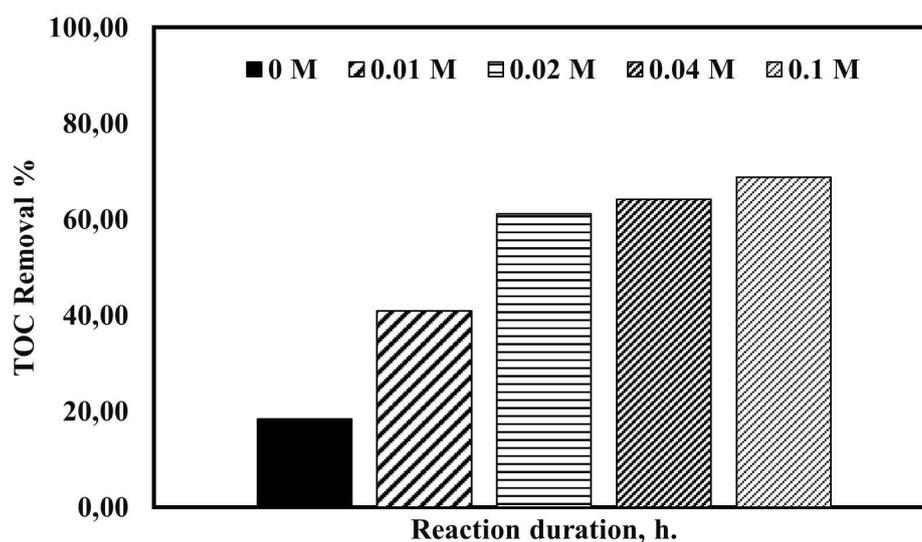
Figure 3. TOC removal % depending on NaOH concentration (*reaction conditions*: 100 ml of sugar industry wastewater,  $T = 180^\circ\text{C}$ ,  $t = 1\text{ h}$ ,  $[\text{NaOH}]_0 = 0\text{--}0.1\text{ M}$ ).
