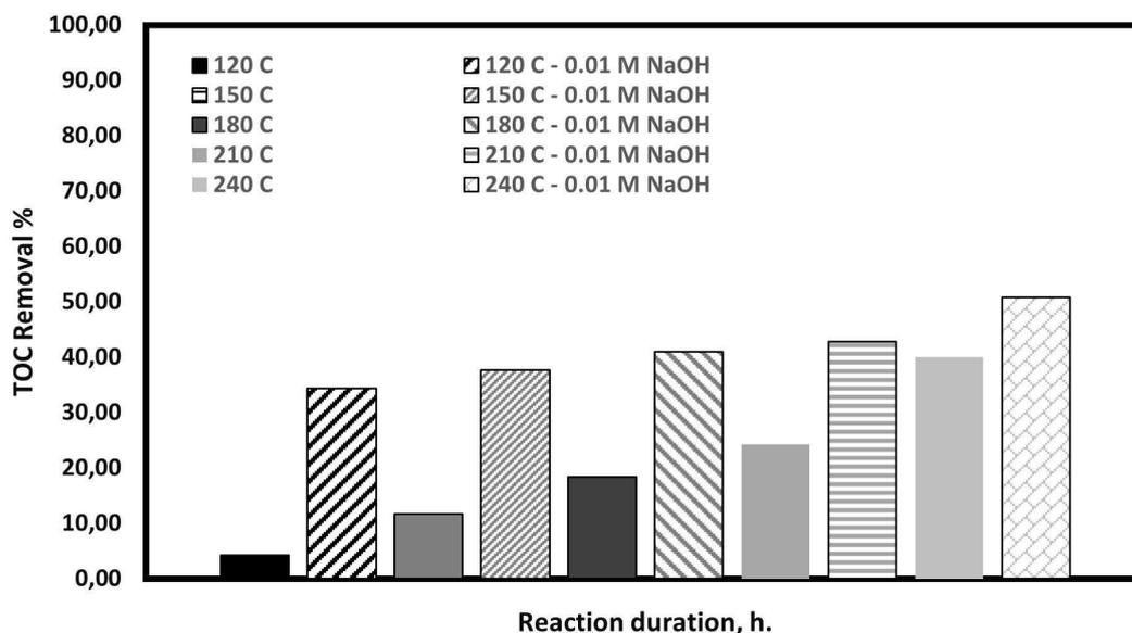
Figure 2. TOC removal % depending on reaction temperature (*reaction conditions*: 100 ml of sugar industry wastewater,  $T = 120\text{--}240^\circ\text{C}$ ,  $t = 1\text{ h}$ ,  $[\text{NaOH}]_0 = 0.01\text{ M}$ ).
