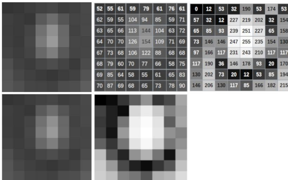
Figure 2. Histogram equalization of a sample 8-bit grayscale 8x8 image, its pixel values and the image before and after the equalization [28]
