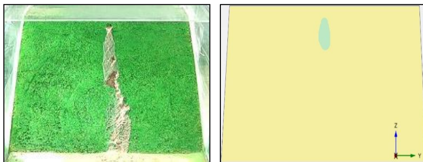
Figure 6.36. The downstream temporal breach developments (a) 0 s, b) 40 s, c) 240 s, d)
