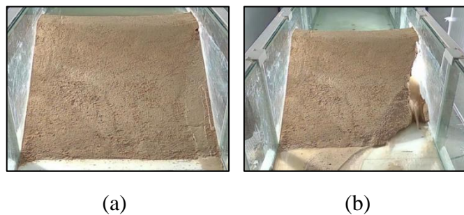
Figure 6.46. The experiment process for the upper-corner scenario (a) downstream beginning (b) downstream ending (c) right side beginning (d) right side ending (e) upstream beginning (f) upstream ending
