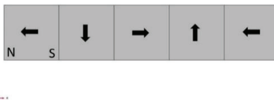
Figure 11. 2D view of the Halbach array design consisting of five neodymium magnets.
