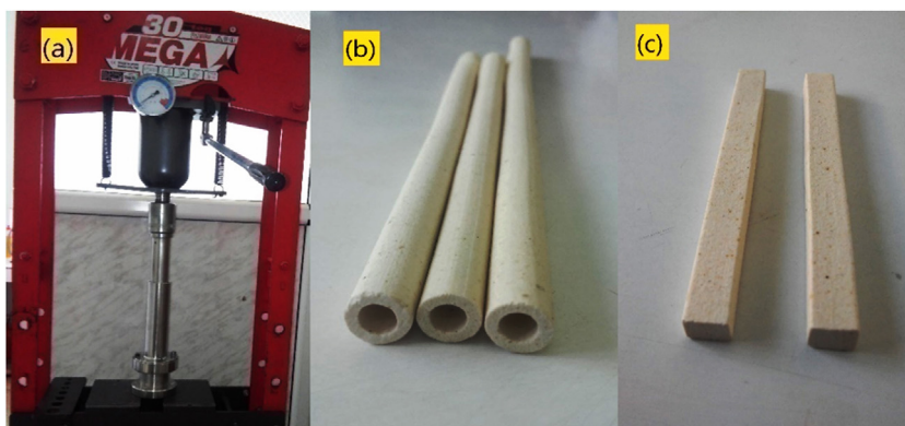
Fig. 1 – (a) A photograph of a mechanical extruder. (b, c) A photograph of prepared tubular and flat rectangular supports, respectively.
