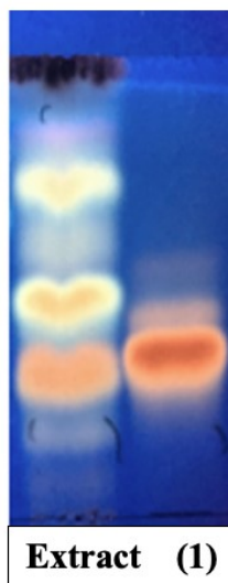
Chromatogram 3.1. Thin layer chromatogram of the EtOAc extract obtained from preparative scale biotransformation study of cyclocephanol by C. laburnicola [Reverse phase C18 silica gel, Mobile phase: 70:30 (ACN: H 2 O)].
