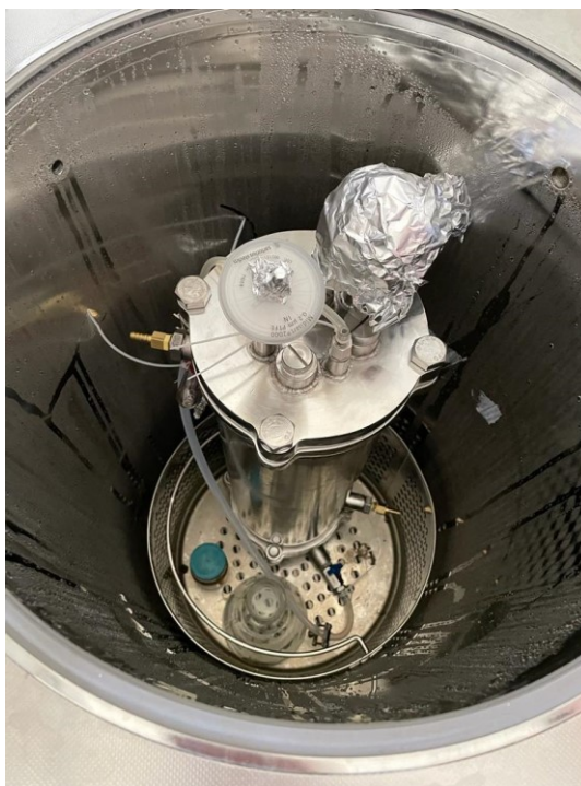
Figure 4.7. Bioreactor ready for sterilization in the autoclave.
