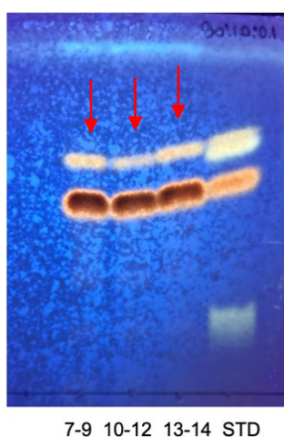
Chromatogram 5.20. Activity test results of the fractions obtained from IEC-2 (Incubation time: 12 h) [Silica gel, Mobile phase: 90:10:0.1 (CHCl 3 :MeOH:H 2 O)].
