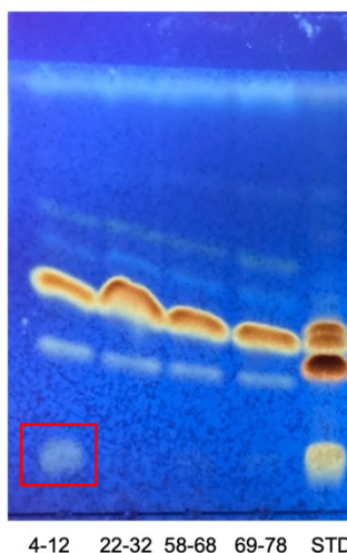
Chromatogram 5.9. Activity test results of the fractions obtained from SEC-1 (Incubation time: 23 h) [Silica gel, Mobile phase: 90:10:0.1 (CHCl 3 :MeOH:H 2 O)].
