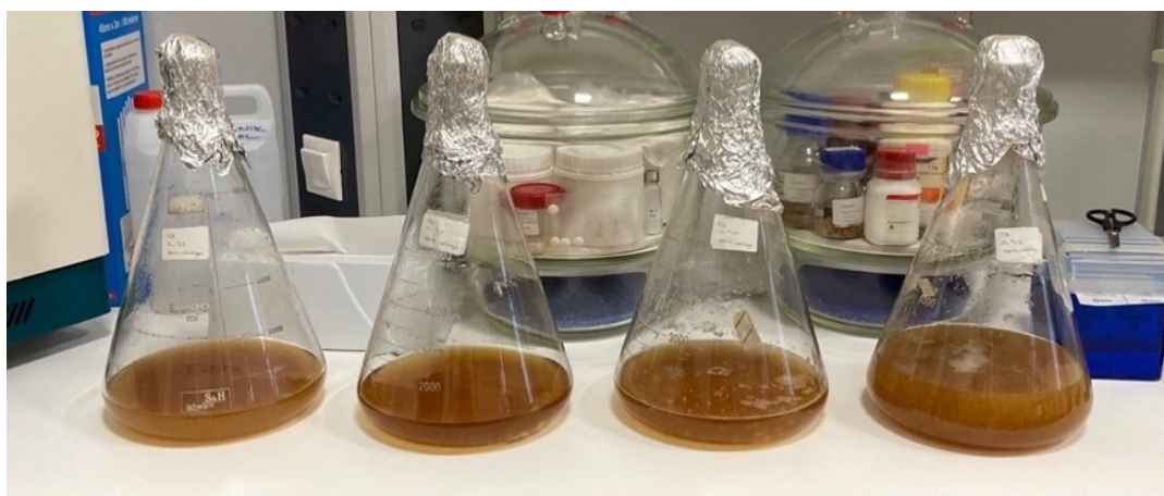
Figure 4.5. 5 L shake flasks used in microbial biotransformation studies.
