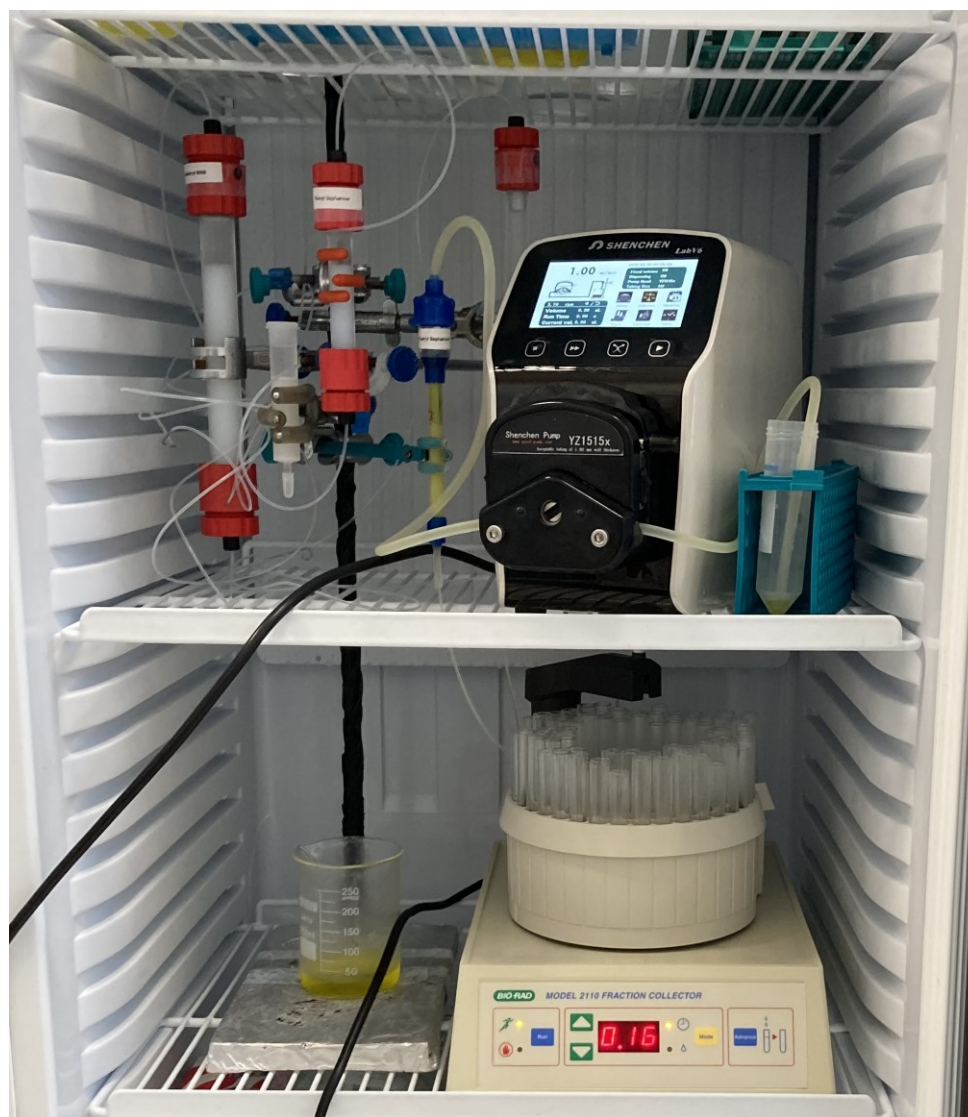
Figure 5.11. Low-pressure liquid chromatography system installed for chromatographic processes.
