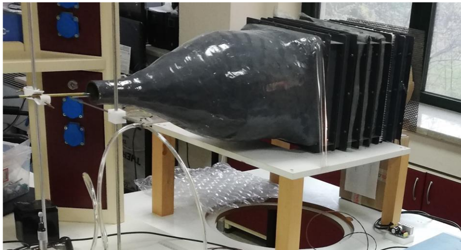
Figure 3.19: Jet flow nozzle for experiments (Source: Arıdıcı, 2022)
