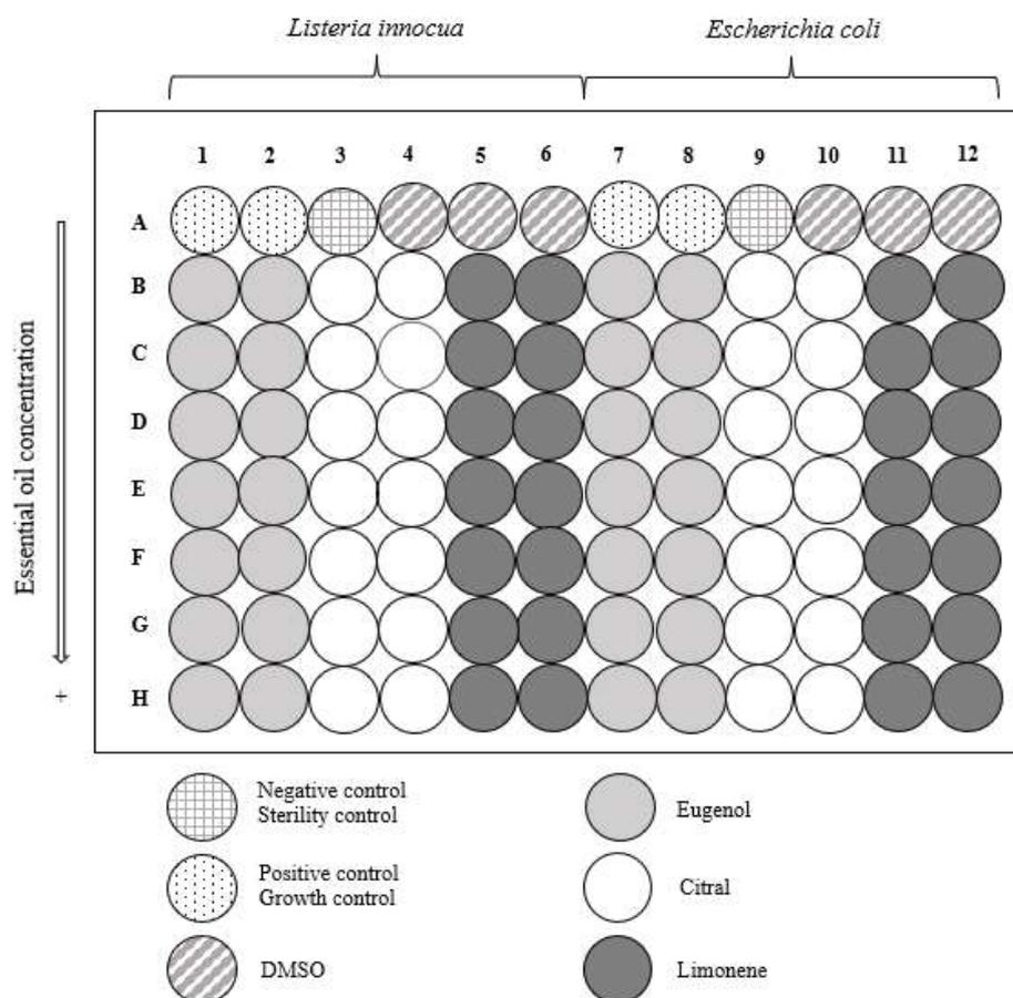
Figure 2.2. Experimental design for determining minimum inhibitory concentration (MIC) of three different essential oils: eugenol, citral, limonene.
