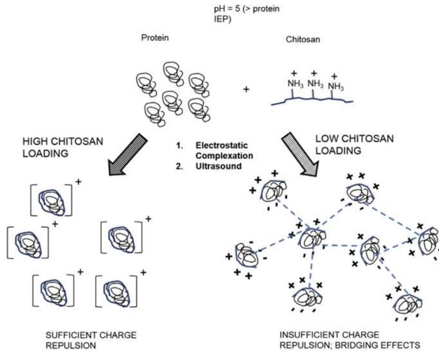
Figure 2.4. Types of complexes that can be produced by the complexation of chitosan and protein: coacervate or droplets (left-side) (liquid-liquid phase separation) and solid precipitate or particles (right-side) (liquid-solid phase separation) (Source: Kurukji, Norton, and Spyropoulos 2016).
