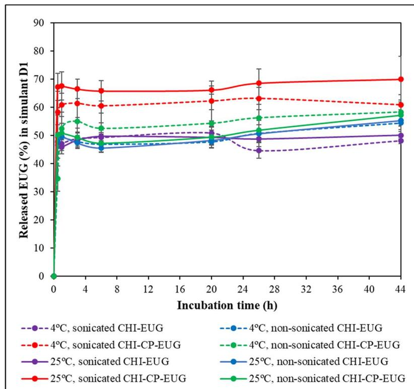
Figure 2.7. EUG release profiles of films during incubation in simulant D1 (50% ethanol) at 4°C and 25°C.
