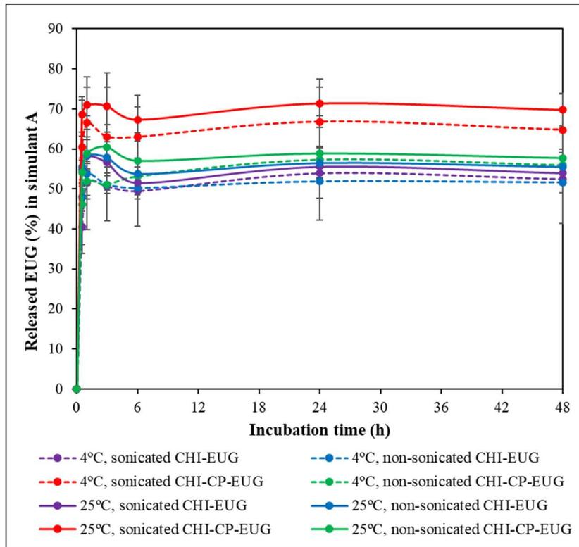
Figure 2.6. EUG release profiles of films during incubation in simulant A (10% ethanol) at 4°C and 25°C.
