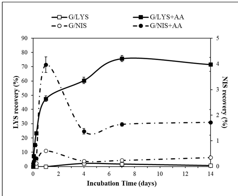
Figure 1.3. LYS (primary y-axis) and NIS (secondary y-axis) release profiles of GEL/SP/IN/SUC gels (G) with or without ascorbic acid (AA) during incubation in distilled water at 4°C.
