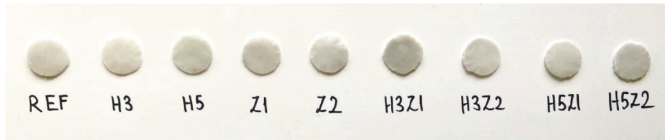
Figure 3.9 Water sorption and solubility test specimens
