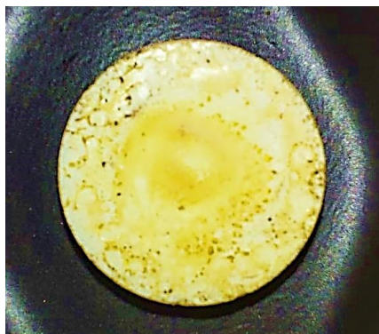
Figure 4.1. An example photograph of a MgAl 2 O 4 spinel coated alumina pellet.
