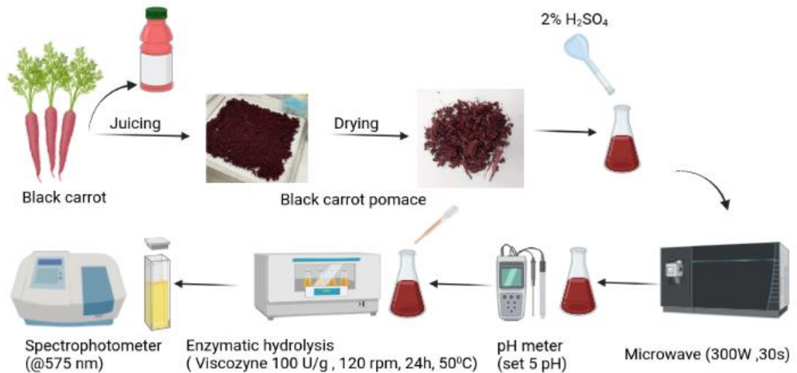
Figure 3. Schema of microwave assisted diluted acid pretreatment
