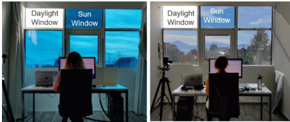
Figure 2.2. Blue tinted (left) and clear glazing(right) used for the experiment (Source: Jain et al. 2023)
