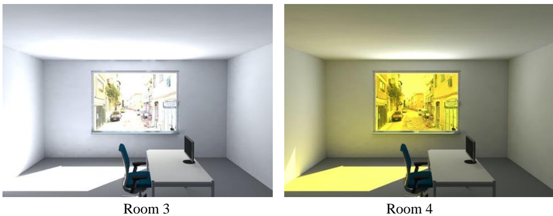
Figure 4.8. Rooms with the most (left) and least (right) indoor brightness satisfaction
