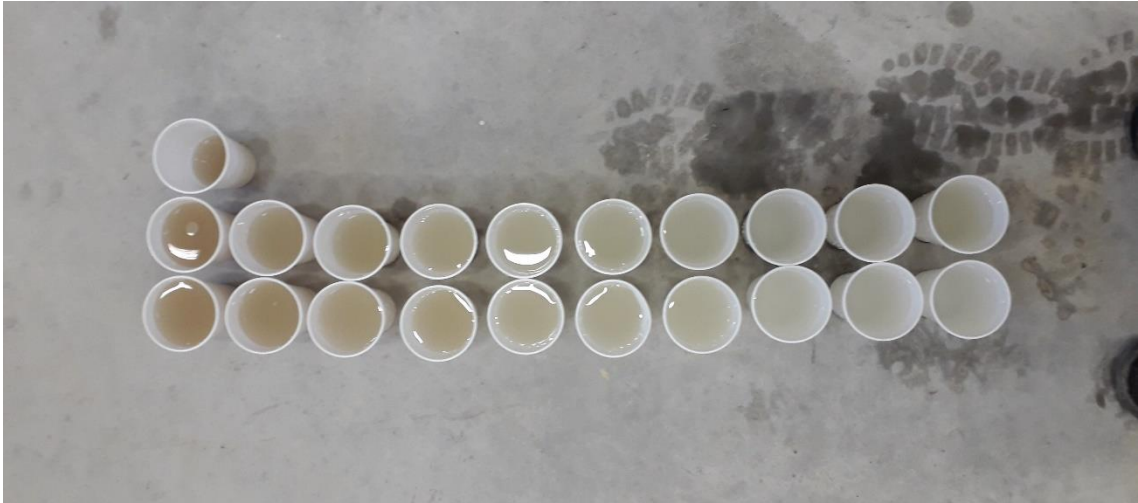
Figure 3.8 Change of water quality for the filter with FC of 0% (Source: Ecemis, 2023)
