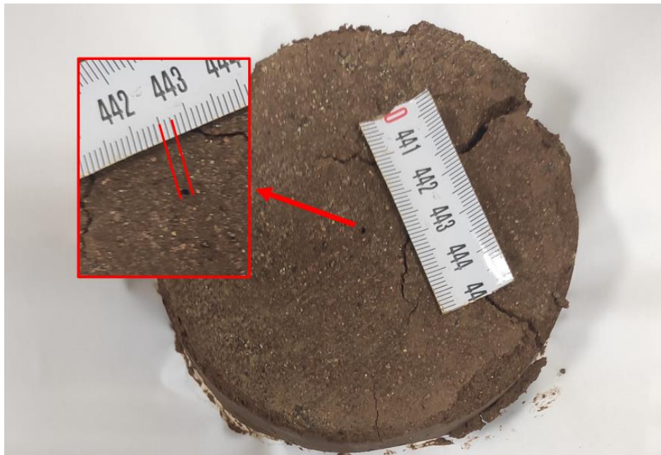
Figure 3.20 Final hole diameter for 2Hz frequency dynamic test (Source: Ecemis, 2023)
