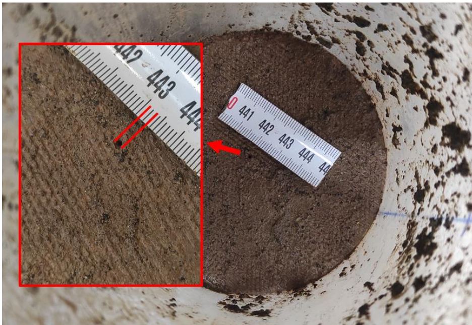
Figure 3.15 Final hole diameter (1 mm) for the filter with FC of 5% (Source: Ecemis, 2023)
