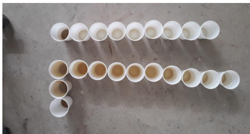
Figure 3.22 Change of water quality for 4Hz frequency dynamic test (Source: Ecemis, 2023)
