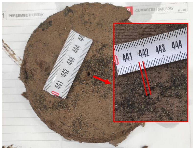
Figure 3.9 Final hole diameter (2 – 3 mm) for the filter with FC of 0% (Source: Ecemis, 2023)
