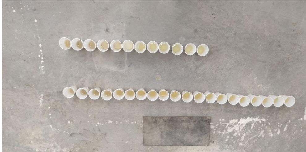
Figure 3.19 Change of water quality for 2Hz frequency dynamic test (Source: Ecemis, 2023)
