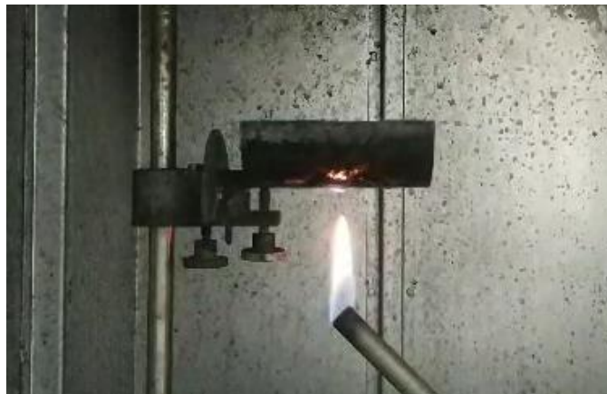
Figure 4.19. Half tube sample during flammability test
