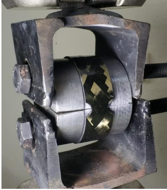
Figure 3.11. Split disk test setup with sectioned ring sample
