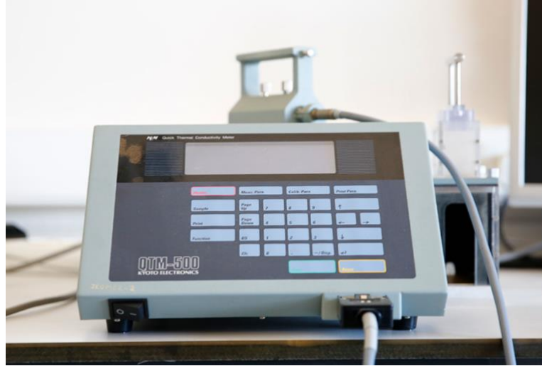
Figure 3.18. Thermal conductivity meter test equipment (QTM 500)
