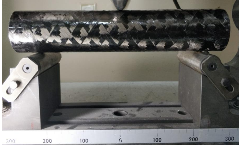
Figure 3.15. Test setup of 3-point bending test
