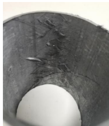
Figure 4.9. The close-up image of fiber damage after radial compression test
