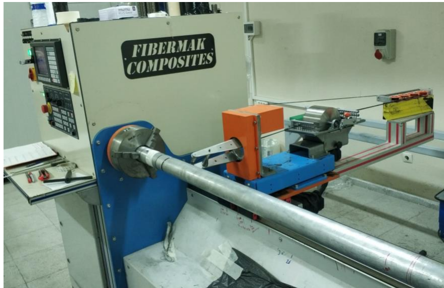
Figure 3.2. Filament winding machine and the setup for composite tube
