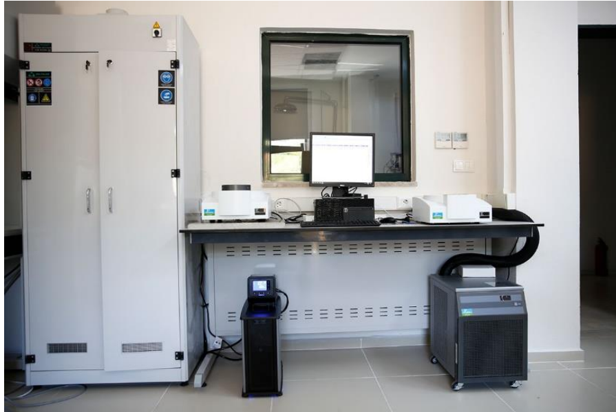
Figure 3.16. PerkinElmer Diamond (TG/DTA) system
