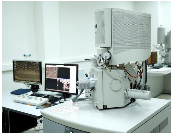
Figure 3.22. SEM test equipment (FEI QUANTA 250 FEG)
