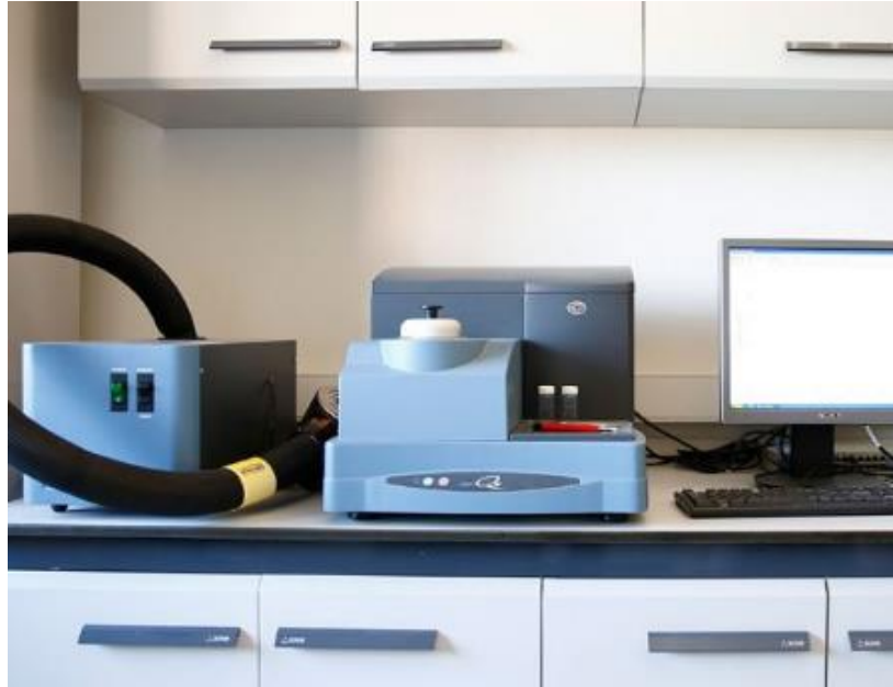
Figure 3.17. DSC test equipment (TA Instruments Q10)
