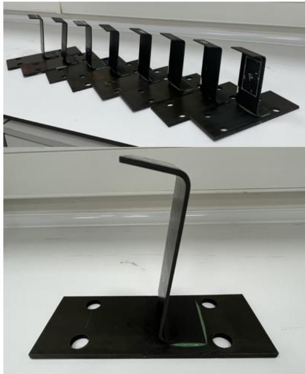
Figure 32. SSJ test specimens.
