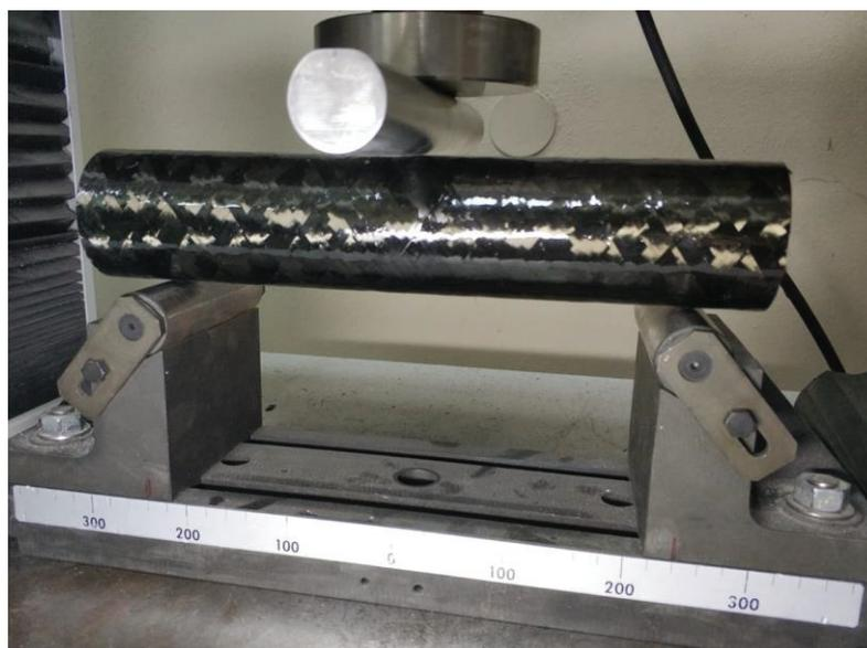
Figure 27. Three-point bending test setup.
