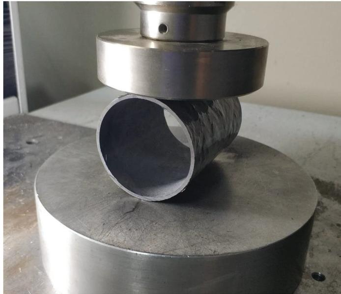
Figure 29. Radial compression test setup.
