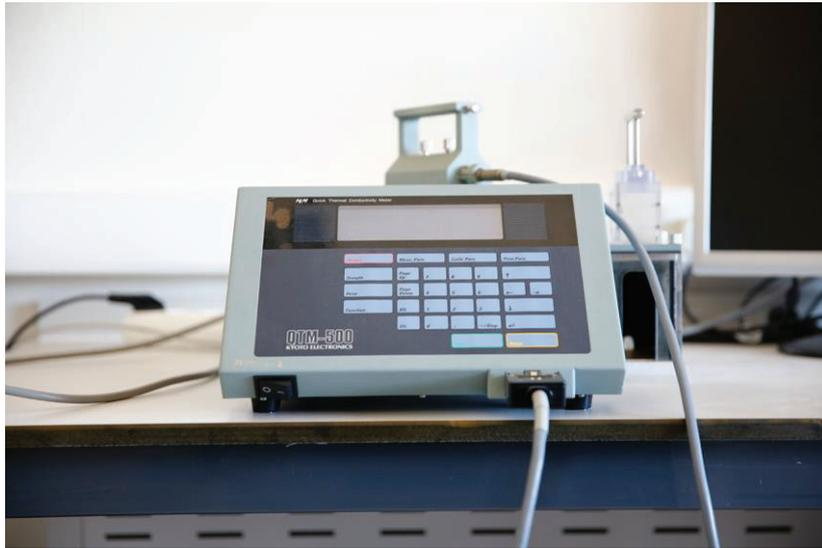
Figure 26. KEM QTM 500 Thermal conductivity meter.
