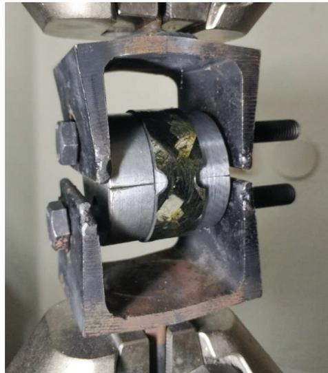
Figure 28. Hoop tensile test setup.
