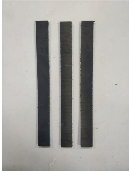
Figure 24. The Combined Loading Test Specimens.
