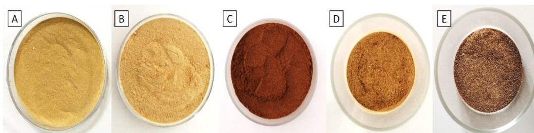
Figure 3.4. Photographic images of commercial pectins and different fig pectins: [citrus pectin (CP) (A), apple pectin (AP) (B), crude low-grade dried fig pectin (CFP) (C), crude fig stalk pectin (CSP) (D) and purified fig stalk pectin (PSP) (E)].
