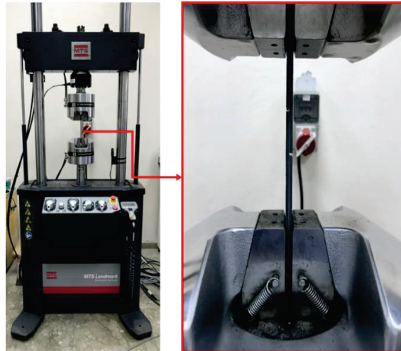
Figure 30. Image of a single lap joints test sample
