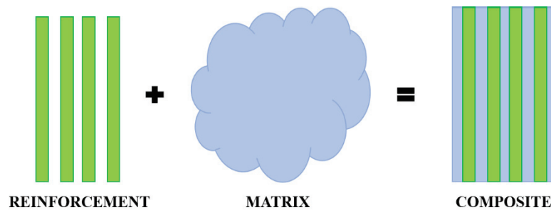
Figure 1. Illustration of the phases of composite materials.
