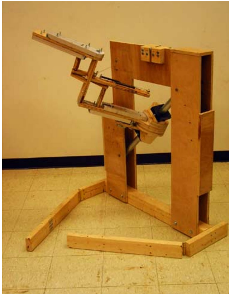
Figure 2.16. Gravity balanced two dof spatial serial manipulator (Source: Agrawal & Fattah, 2004)
