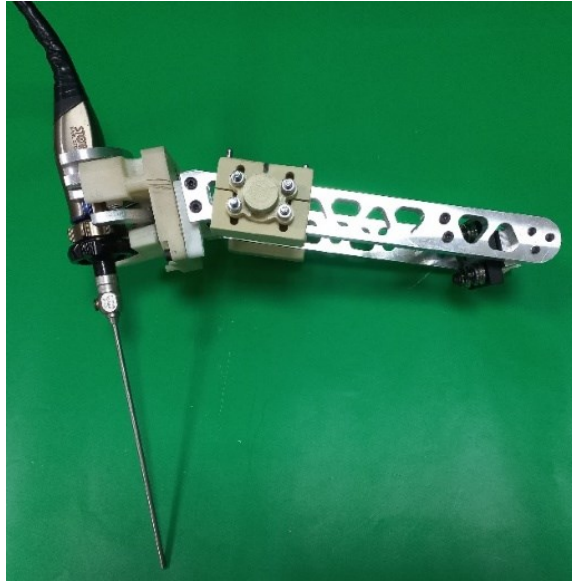
Figure 5.29. Completed assembly of the linear carriage (sub-assembly of D)
