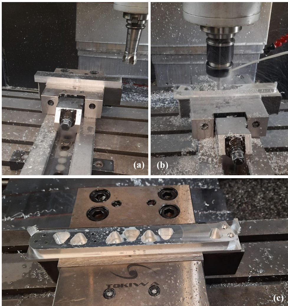
Figure 5.25. Machining process of bridges (a) Fixing raw material on the CNC machine, (b) Machining process of the bridge and (c) After finishing machining on one face
