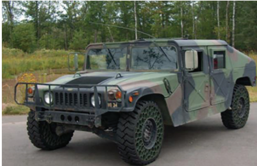
Figure 1.1. One of the usage areas of TPU in the defense industry (Source : “Airless Tyres for Military Humvee” 2021)
