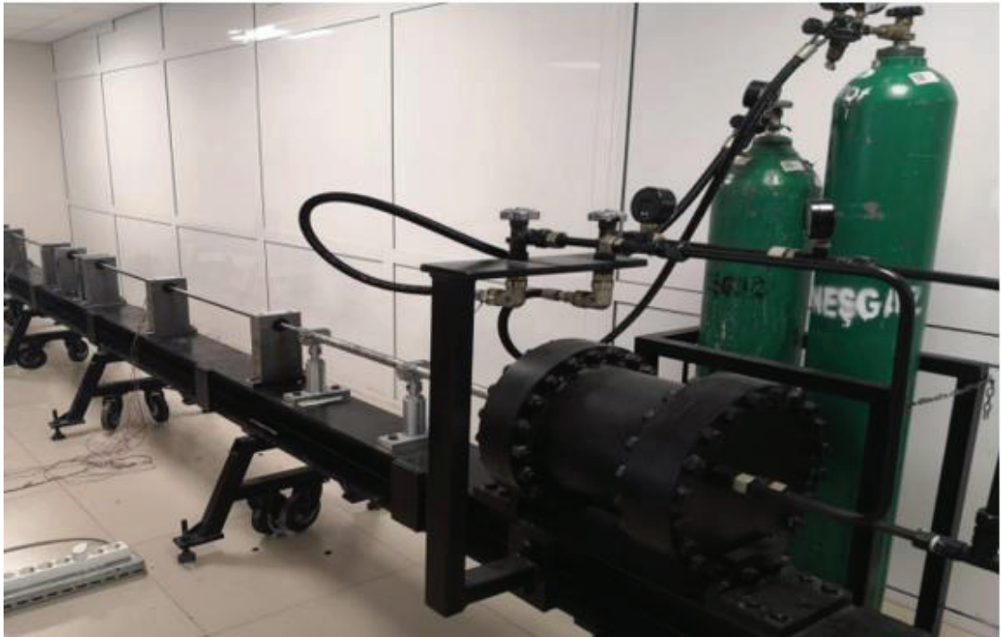
Figure 2.16. Test setup of the Split Hopkinson Pressure Bar
