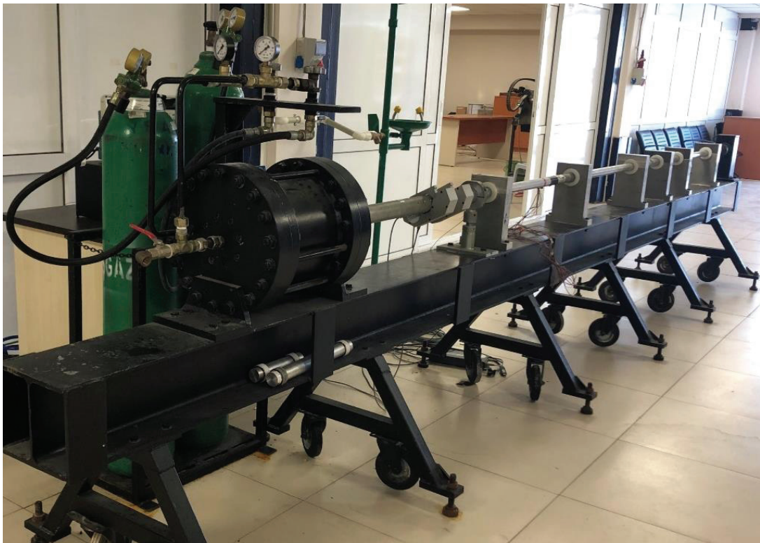
Figure 2.12. Direct impact test setup
