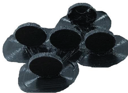
Figure 2.4. Compression cylindrical specimen used for material characterization
