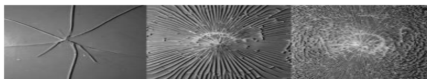
Figure 2.5 Fracture model: annealed-glass, heat strengthened glass, and toughened glass (Source: Haldimann et al. 47 )
