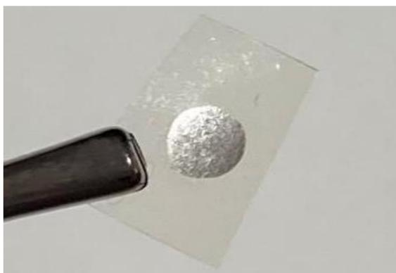
Figure 2.2. Polymer sample with silver paste for electrical measurements.
