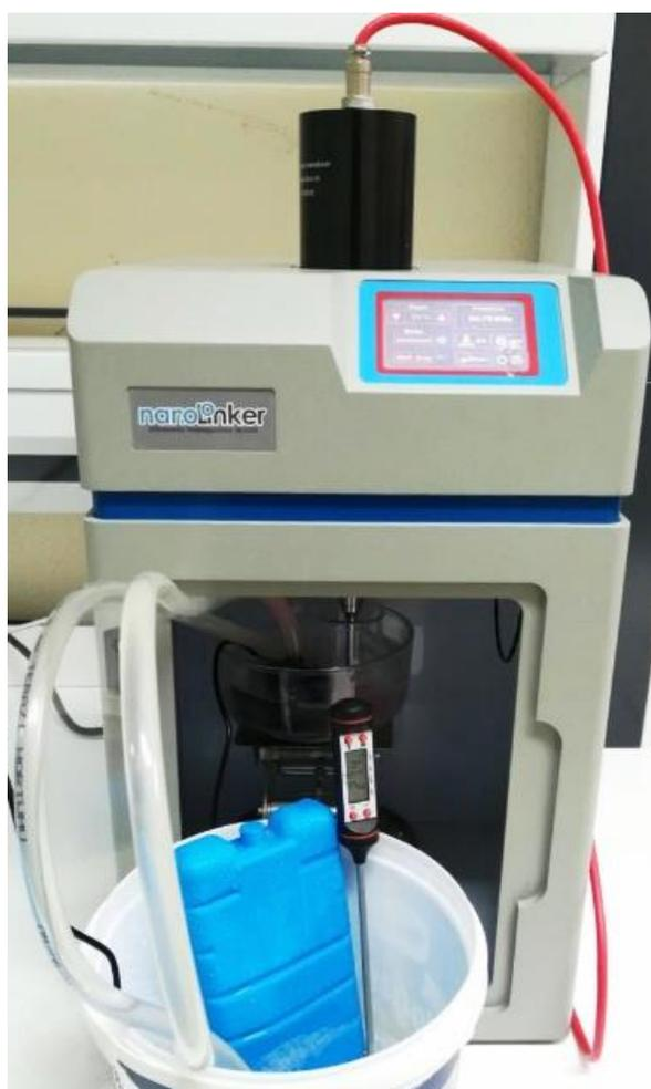
Figure 2.4. Experimental water circulation set-up for the sonicator.
