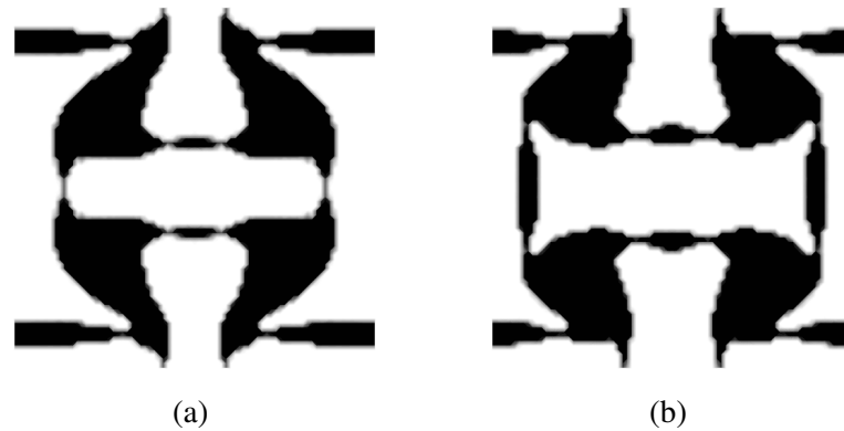
Figure 7.20: (a) The optimum topology of a unit cell optimized for negative Poisson's ratio under linear behavior, (b) Optimum topology of the same unit cell with identical optimization parameters, under nonlinear behavior.
