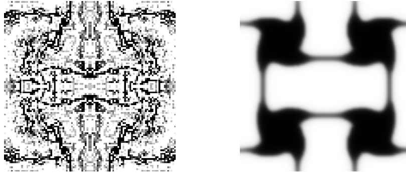
Figure 5.3: Optimum topology of a unit cell optimized without using Helmholtz filter (Left). Optimum topology of the same unit cell, optimized using Helmholtz filter (Right). Both unit cells have been optimized for negative Poisson's ratio under linear analysis, and the domain is discretized into 100 \times 100 mesh.
