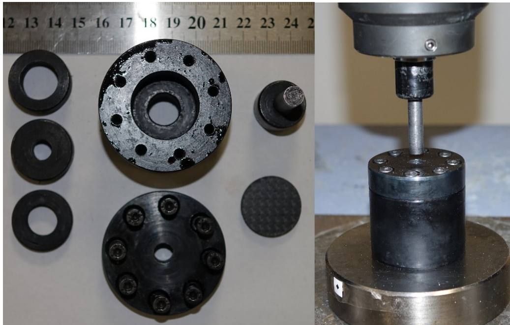
Figure 2.23. Quasi-static Punch Shear test fixture
