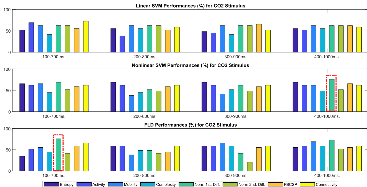
Fig. 5. The recognition performances of our diagnosis framework for CO 2 stimulus. We adopted leave-one-subject-out cross-validation during performance evaluations. We presented the performances for each different time window, feature extraction method, and classifier. The dot-dashed-framed performances indicate the highest ones.
