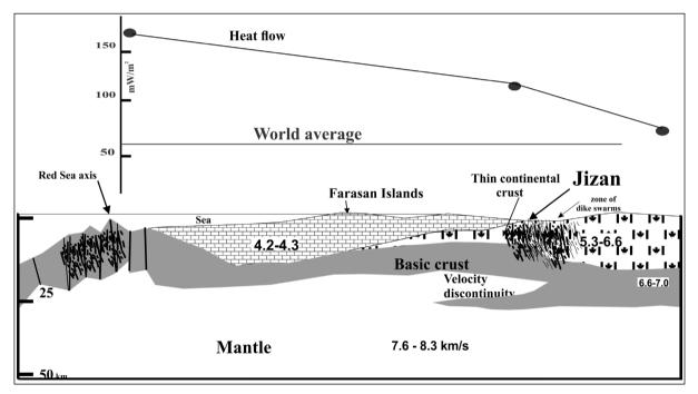
Figure 3- Heat flow and subsurface structure below Jizan, Western Saudi Arabia.
