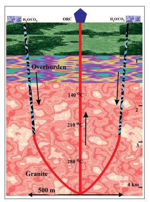
Figure 2- Schematic Closed loop Enhanced Geothermal System model used for THM modeling using COMSOL V6 described in the Section 2.6.
