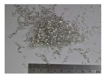
Figure 40. Chip forms of AZ91 alloy at conditions: V<sub>c</sub>:480 m/min, V<sub>f</sub>:0.65 mm/min
