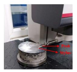
Figure 20. Surface roughness measurement
