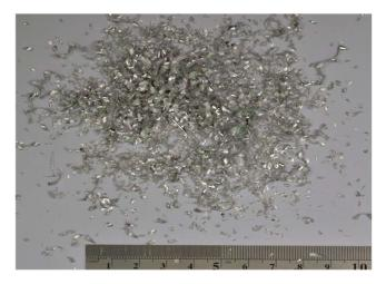
Figure 42. Chip forms of AZ91 alloy at conditions: V<sub>c</sub>:640 m/min, V<sub>f</sub>:0.95 mm/min
