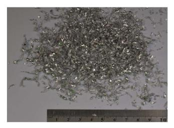
Figure 41. Chip forms of AZ91 alloy at conditions: V<sub>c</sub>:560 m/min, V<sub>f</sub>:0.80 mm/min
