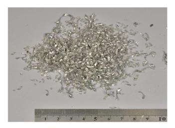
Figure 45. Chip forms of AZ91/2.5 wt.% rCF composite at conditions:  $V_c$ :640 m/min,  $V_f$ :0.65 mm/min
