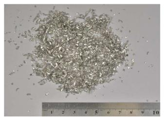
Figure 46. Chip forms of AZ91/5 wt.% rCF composite at conditions:  $V_c$ :480 m/min,  $V_f$ :0.95 mm/min
