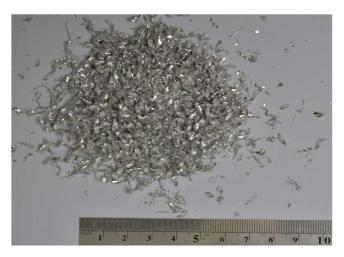
Figure 44. Chip forms of AZ91/2.5 wt.% rCF composite at conditions:  $V_c$ :560 m/min,  $V_f$ :0.95 mm/min
