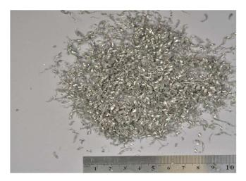
Figure 47. Chip forms of AZ91/5 wt.% rCF composite at conditions:  $V_c$ :560 m/min,  $V_f$ :0.65 mm/min
