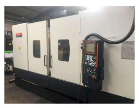
Figure 17. VTC-200C II / Yamazaki Mazak vertical machining device available in TOTOMAK company
