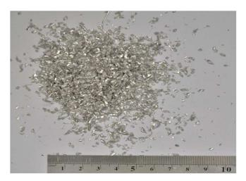
Figure 48. Chip forms of AZ91/5 wt.% rCF composite at conditions:  $V_c\hbox{:}640$  m/min,  $V_f\hbox{:}0.80$  mm/min
